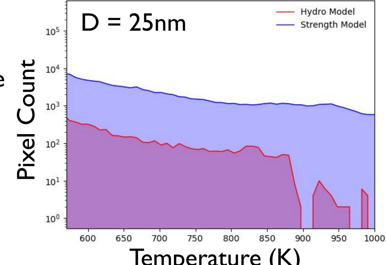
(right) Differences in temperature distributions for  $U_p = 0.75$  km/s and pore sizes 25nm and 2um at a time of 100% pore collapse. Excess temperature from SGL strength model over purely hydrodynamic one manifests in viscous (shear) heating. This extra energy could result in a critical hotspot with a reactive burn model.
