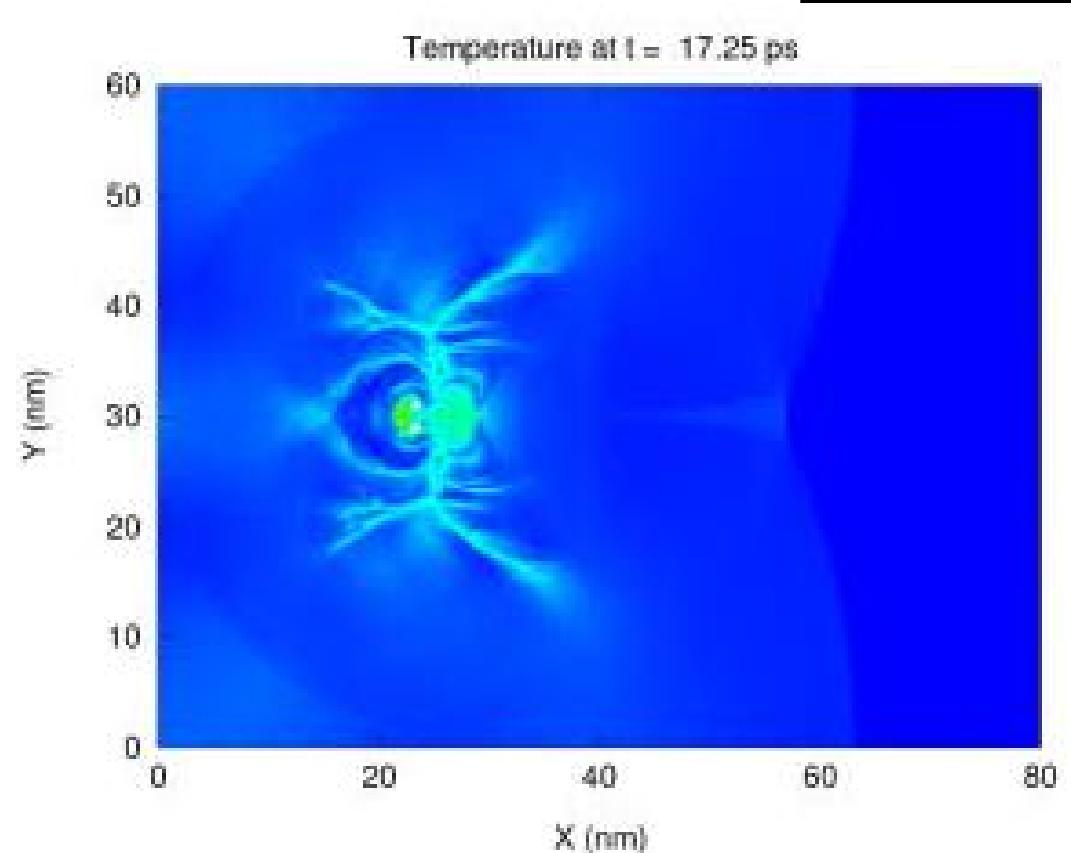
(left) Snapshot of  $U_p = 0.75$  km/s at 100% pore collapse for a 25nm diameter pore. Note the existence of localized shear bands with temperatures above the bulk value as a result of modeling with a strain-rate dependent strength model.
