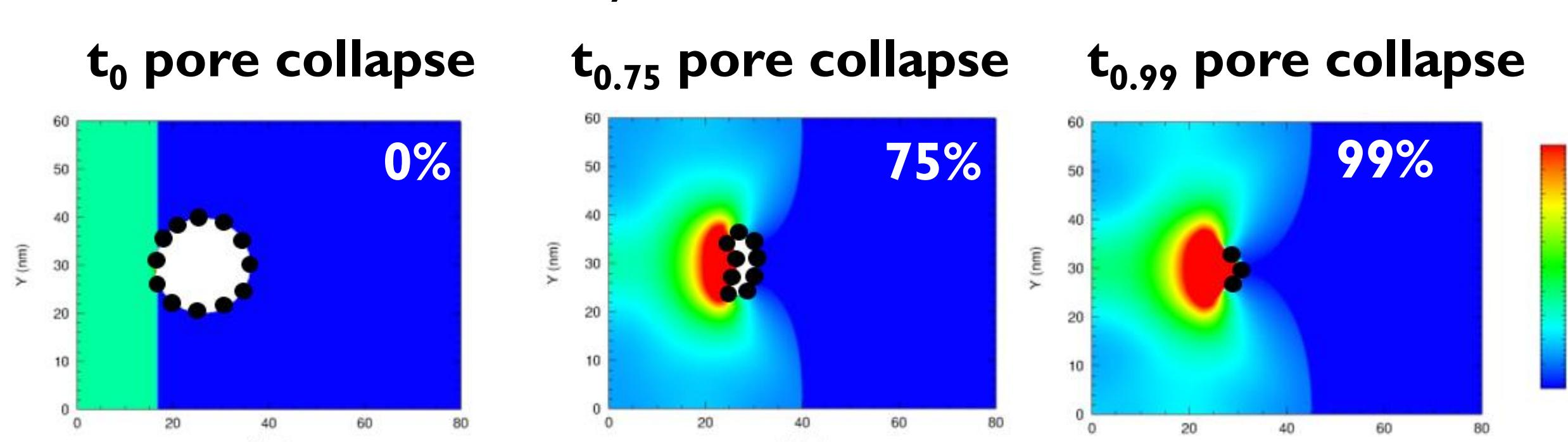
(above) Pore collapse can capture the net effects of material strength
