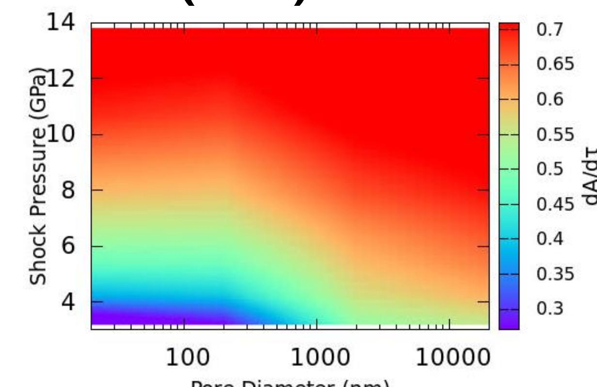
(top) Shock Pressure – Pore Diameter parameter space for pore collapse rate using the MD-informed SGL strength model. Note the relatively larger gradient as a function of shock strength, as compared to pore size
