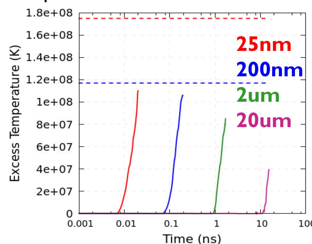
(left) Temperature difference between the SGL and hydrodynamic model captured over time for different pore sizes (solid). Dashed horizontal lines are predictions using Perry et al.<sup>2</sup> critical hotspot theory, where the same color crossover indicates when the strength model would result in a self-sustained deflagration.
