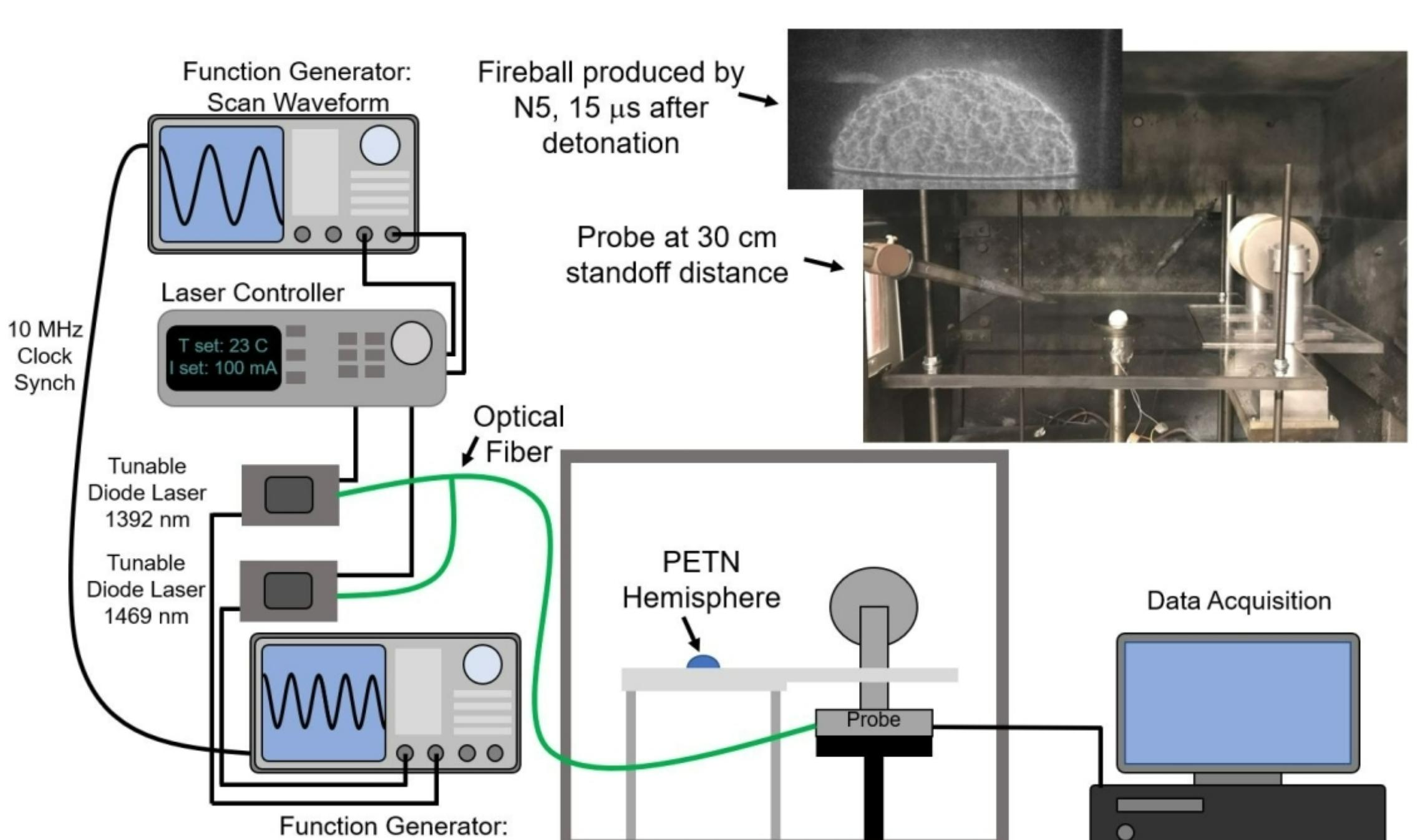
Left: Schematic of setup used to measure  $T$ , and  $H_2O$  in large-scale post-detonation fireballs
