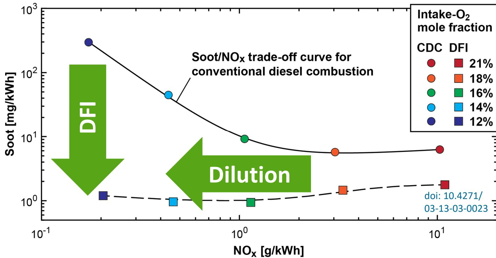
\*Optical-engine results for ~6.8 bar gross indicated mean effective pressure, 1200 rpm, steady state, 4-hole injector, No. 2 diesel fuel
