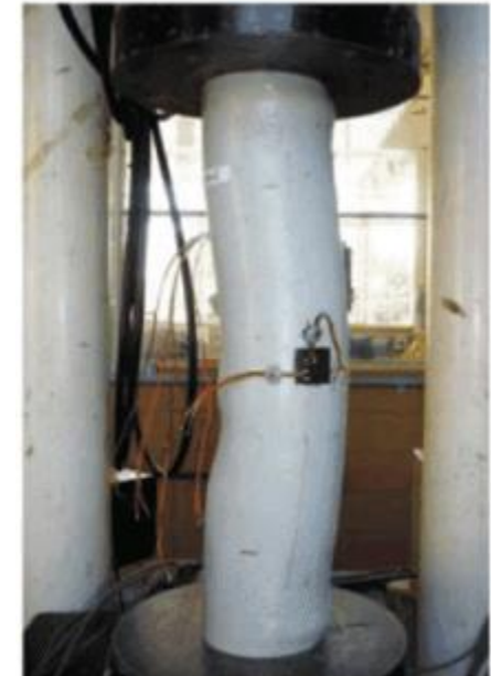
Buckling of a column image: Klimchik www.researchgate.net/figure/Examples-of-buckling-in-column-www-civildb-www-highline_fig11_281183936
