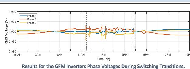
Results for the GFM Inverters Phase Voltages During Switching Transitions.
