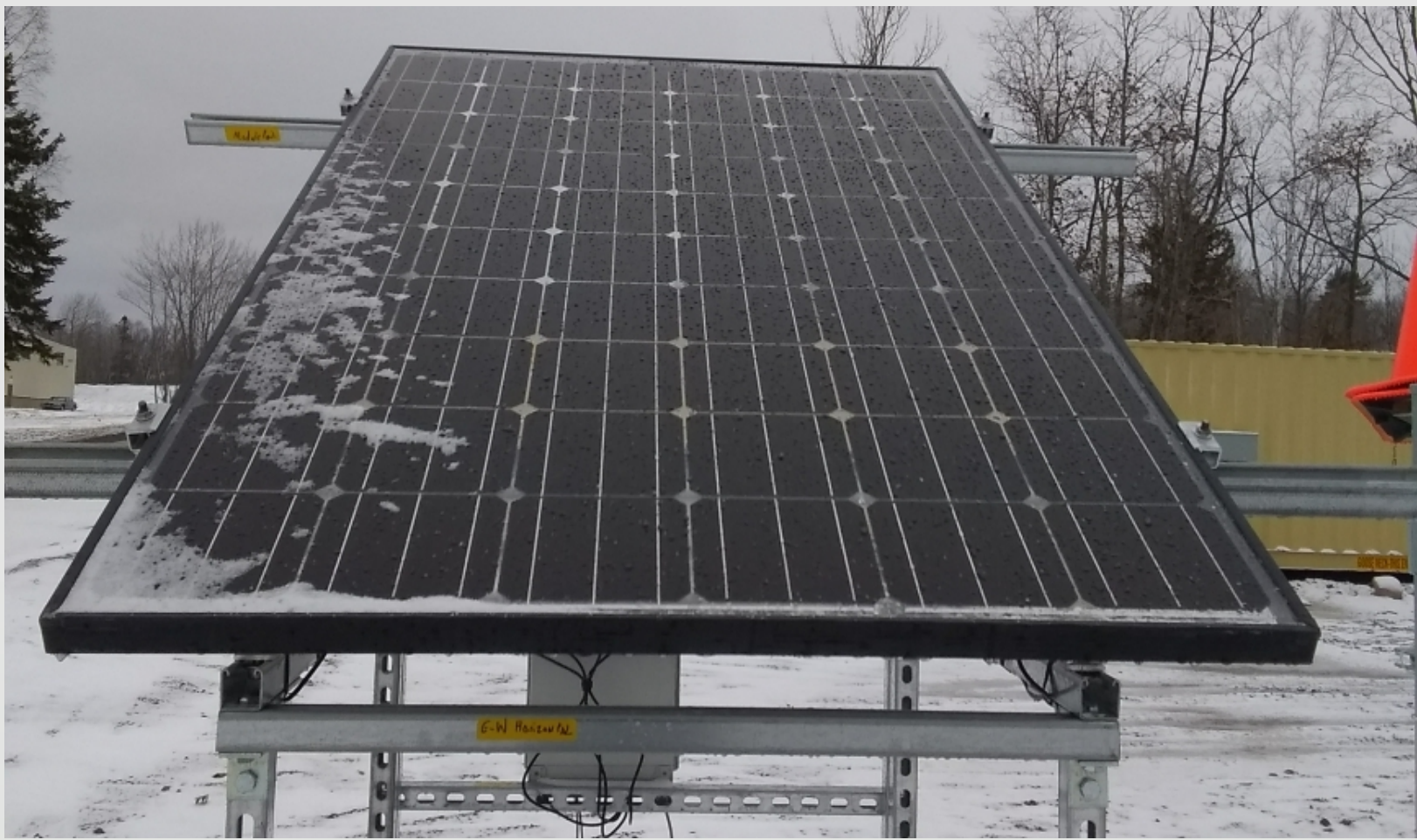
The snow load measurement station installed in 2021.
