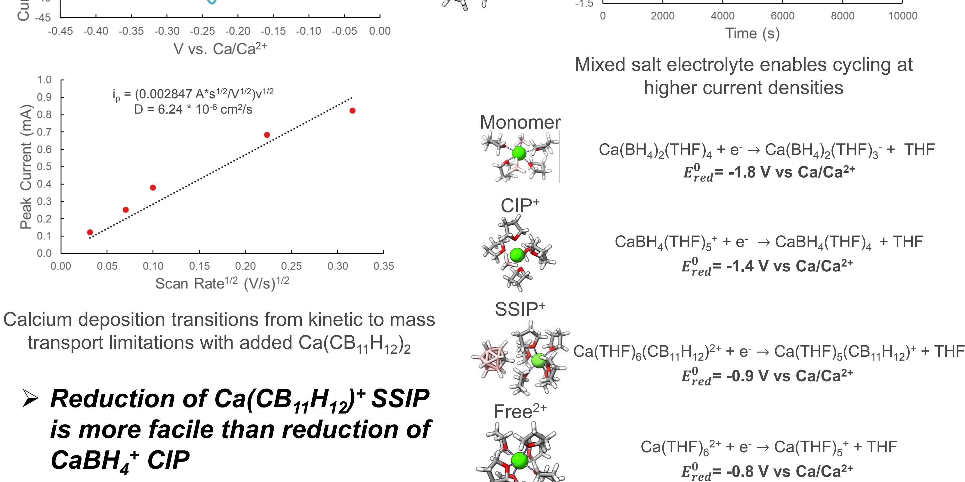
Calcium deposition transitions from kinetic to mass transport limitations with added  $\text{Ca}(\text{CB}_{11}\text{H}_{12})_2$
