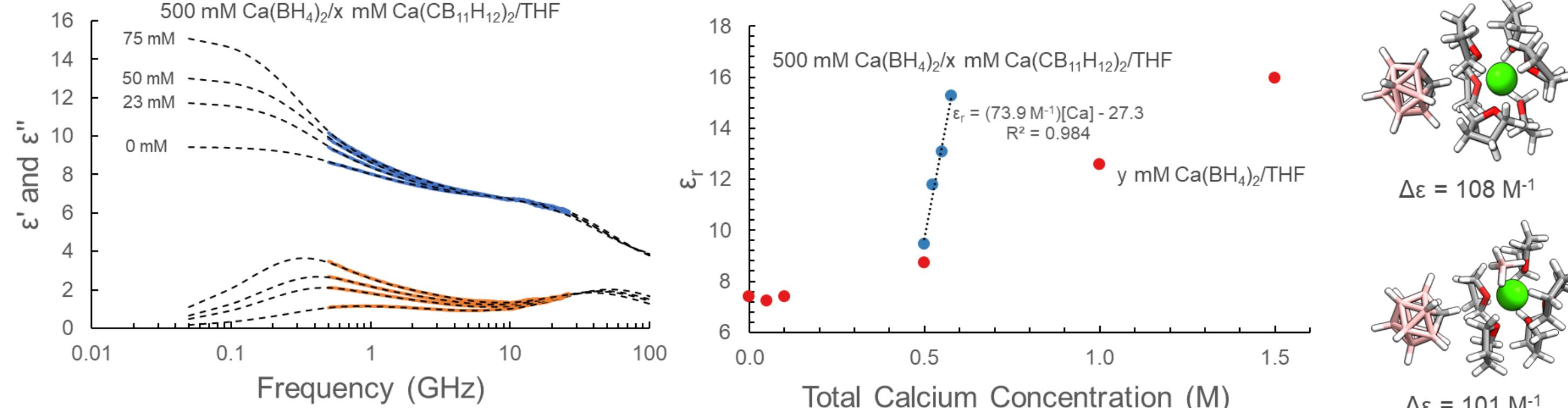
Dielectric relaxation spectroscopy identifies SSIPs as key components of electrolyte
