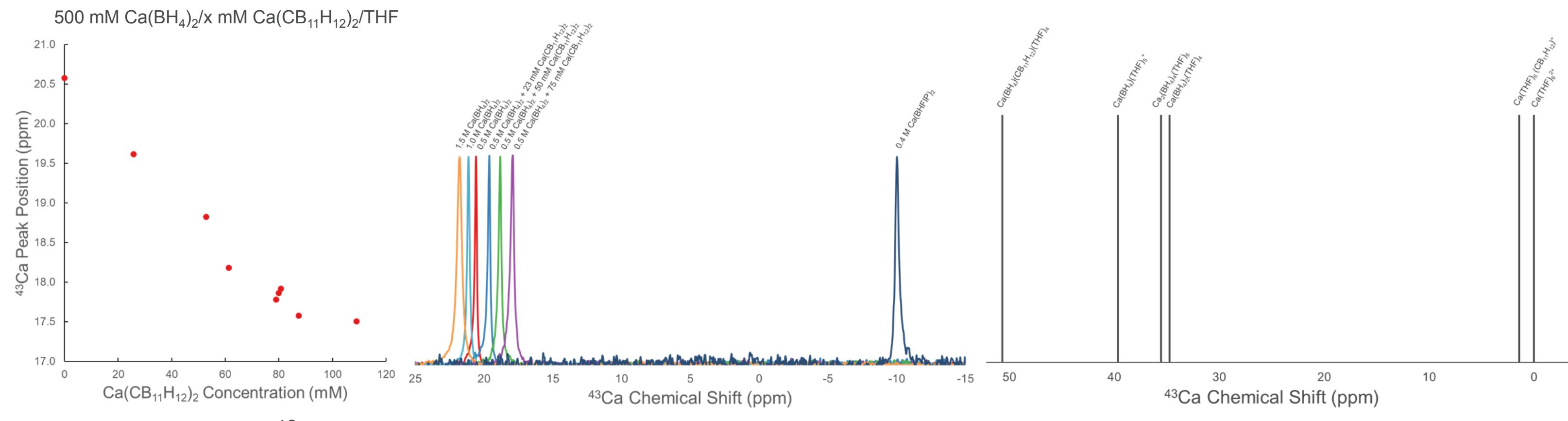
➤ **Addition of  $\text{Ca}(\text{CB}_{11}\text{H}_{12})_2$  to  $\text{Ca}(\text{BH}_4)_2/\text{THF}$  produces  $\text{Ca}(\text{CB}_{11}\text{H}_{12})^+$  SSIPs as alternative  $\text{Ca}^{2+}$  delivery species**
