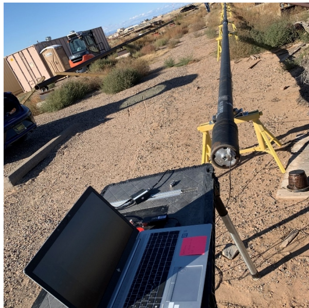
Figure 7: Testing communications with the ethernet-to-coax module through the wired pipe.
