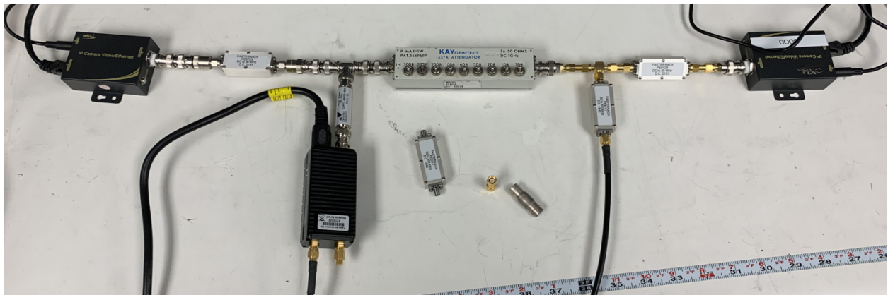
Figure 8: Bench top setup for testing communications and power transfer simultaneously. Variable attenuator represents the wired pipe.
