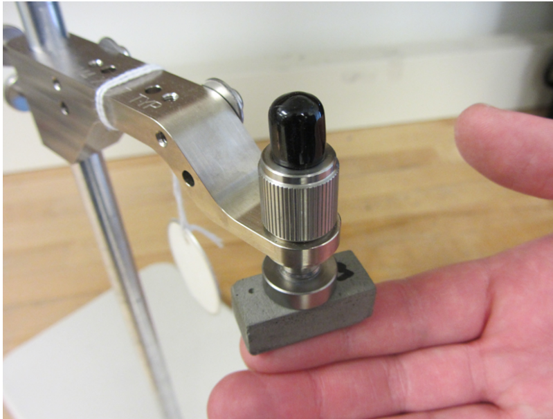
Figure 12: Characterizing the dielectric constant and loss tangent of cement that will be used in the casing annulus.
