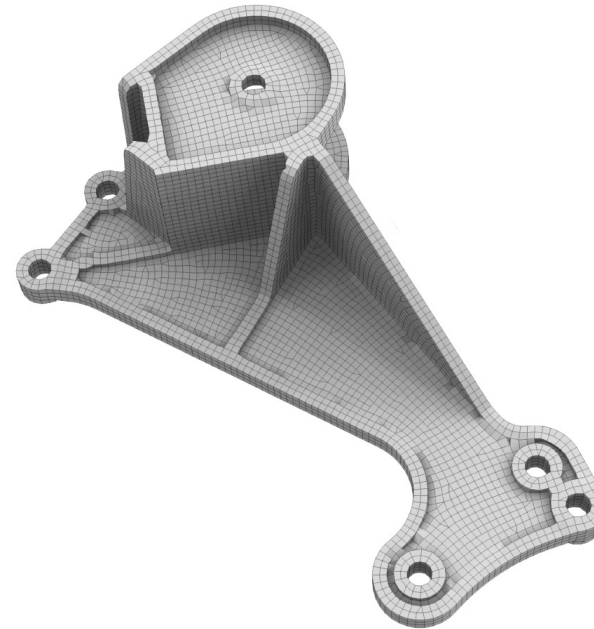
hex-dominant meshing using frame field
