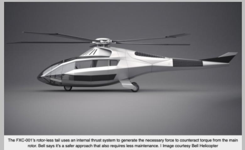
The FXC-001's rotor-less tail uses an internal thrust system to generate the necessary force to counteract torque from the main rotor. Bell says it's a safer approach that also requires less maintenance. | Image courtesy Bell Helicopter
