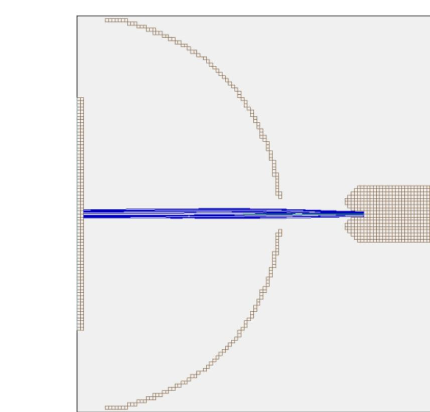
FIG 2.1a: SIMION electron beam simulation, sample Bias = +93VDC, Beam Energy = 30eV
