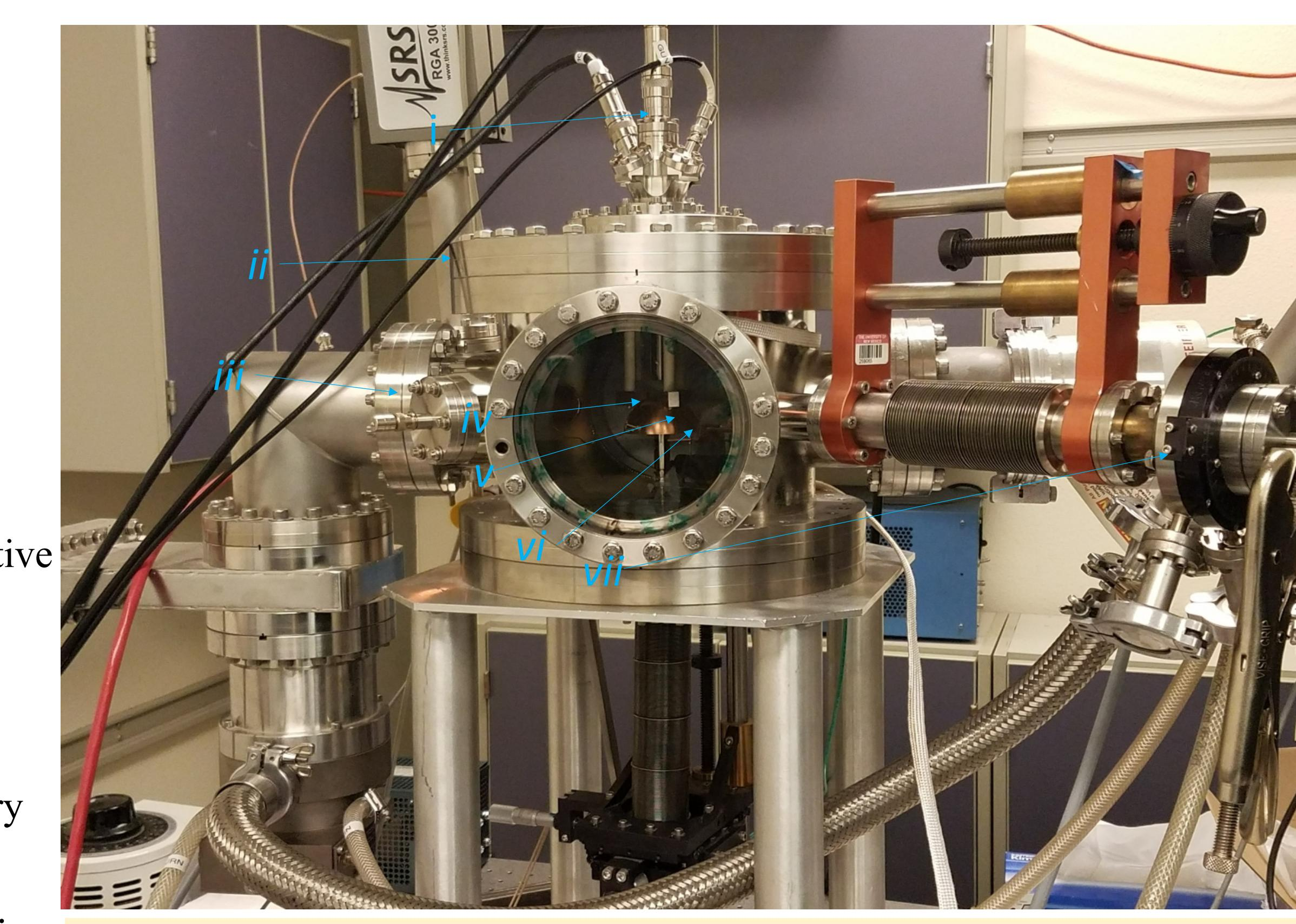
FIG 3.1a: i: Electron Gun, ii: Vacuum Chamber, iii: HCC Measurement Feedthrough, iv: HCC, v: Sample, vi: Sample Holder, vii: Angular Manipulator
