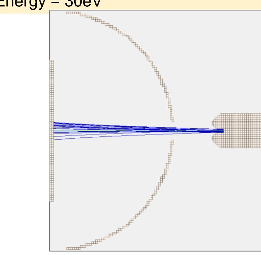
FIG 2.1c: SIMION electron beam simulation: sample bias = -20VDC, beam energy = 30eV.
