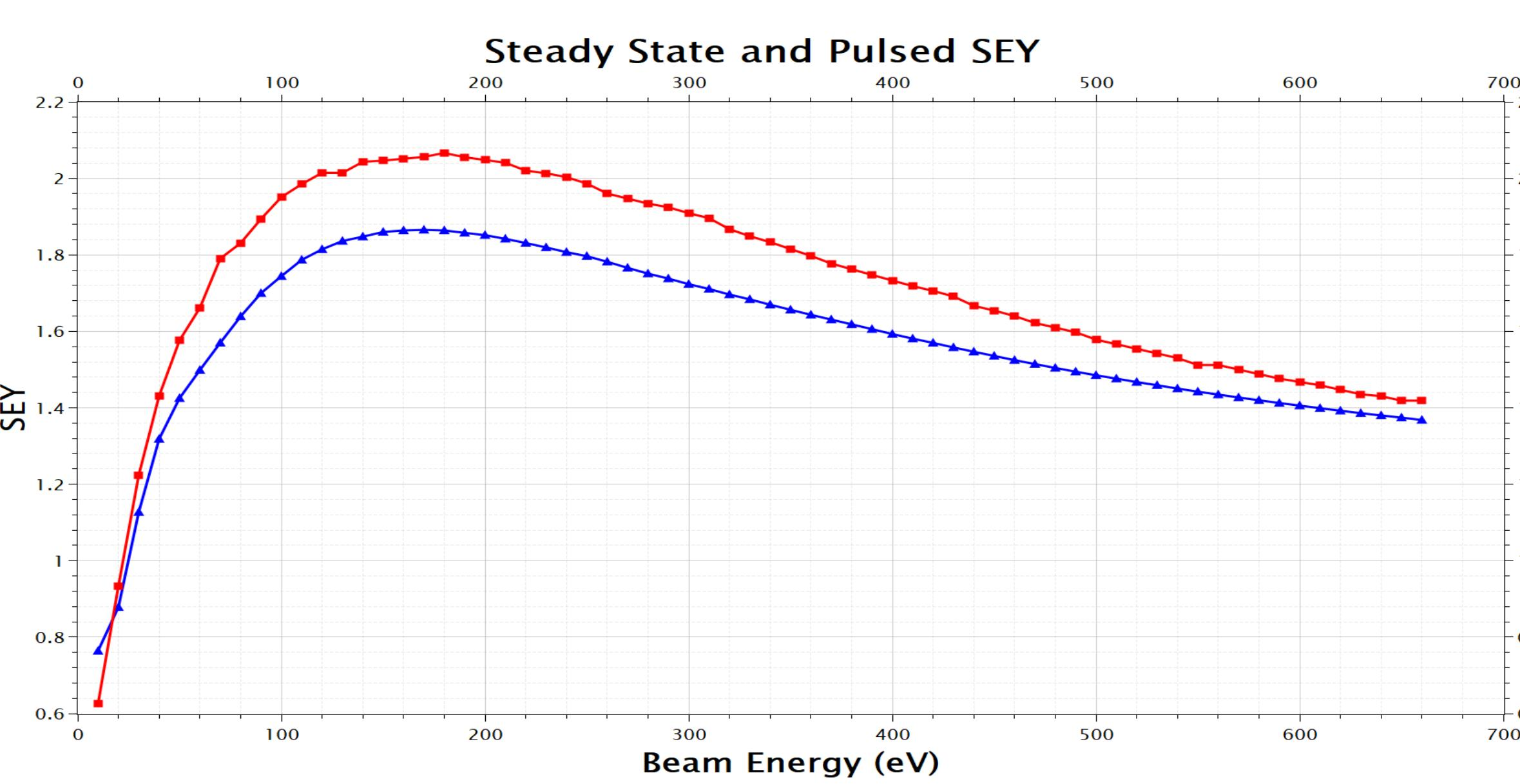
FIG 4.1b: Pulsed Measurement of SEY via HCC (Red) versus Steady-State Measurement of SEY via HCC (Blue)
