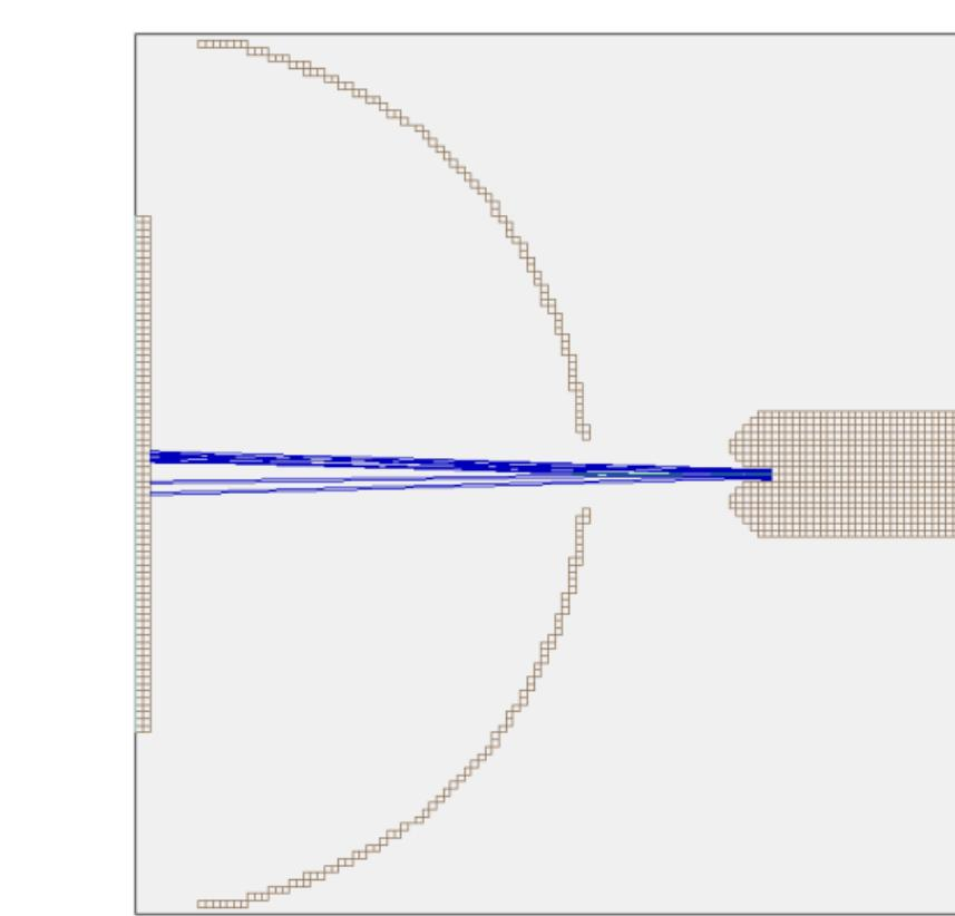
FIG 2.1b: SIMION electron beam simulation, sample bias = +93VDC, Beam Energy = 1000eV
