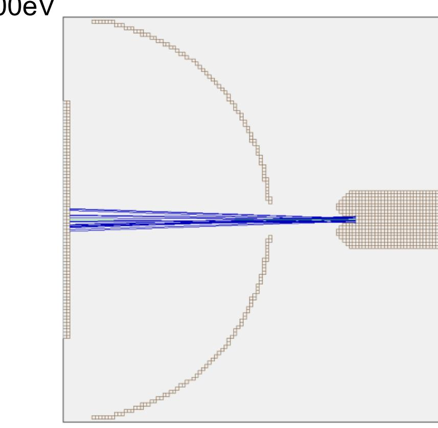
FIG 2.1d: SIMION electron beam simulation, sample bias = -20VDC, beam energy = 1020eV.
