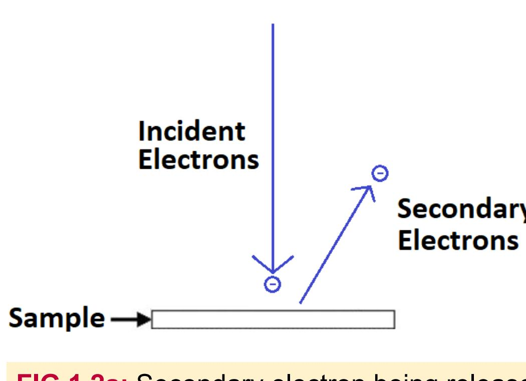
FIG 1.2a: Secondary electron being released
