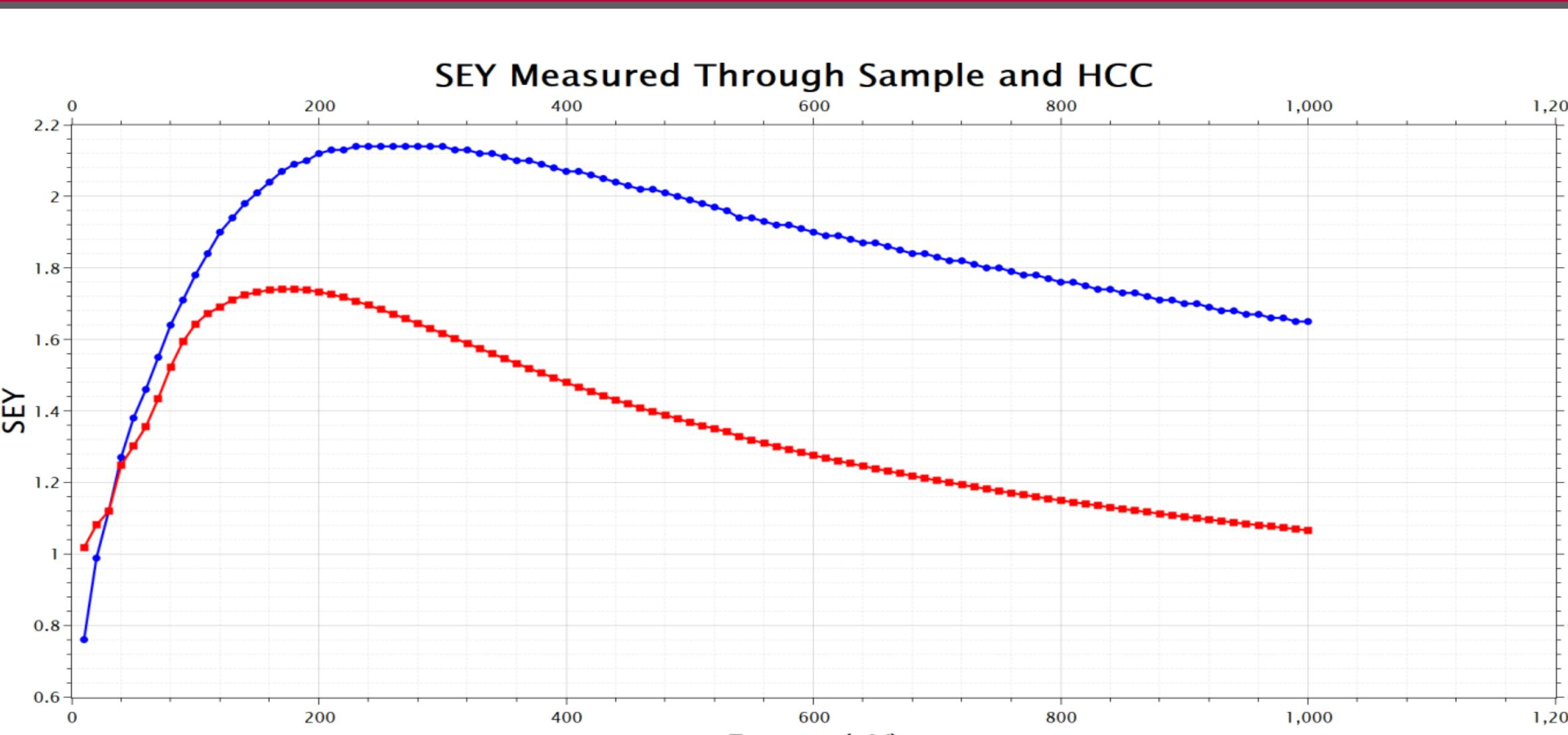
FIG 4.1a: SEY of Copper Sample without the HCC (Blue) and with the HCC (Red).
