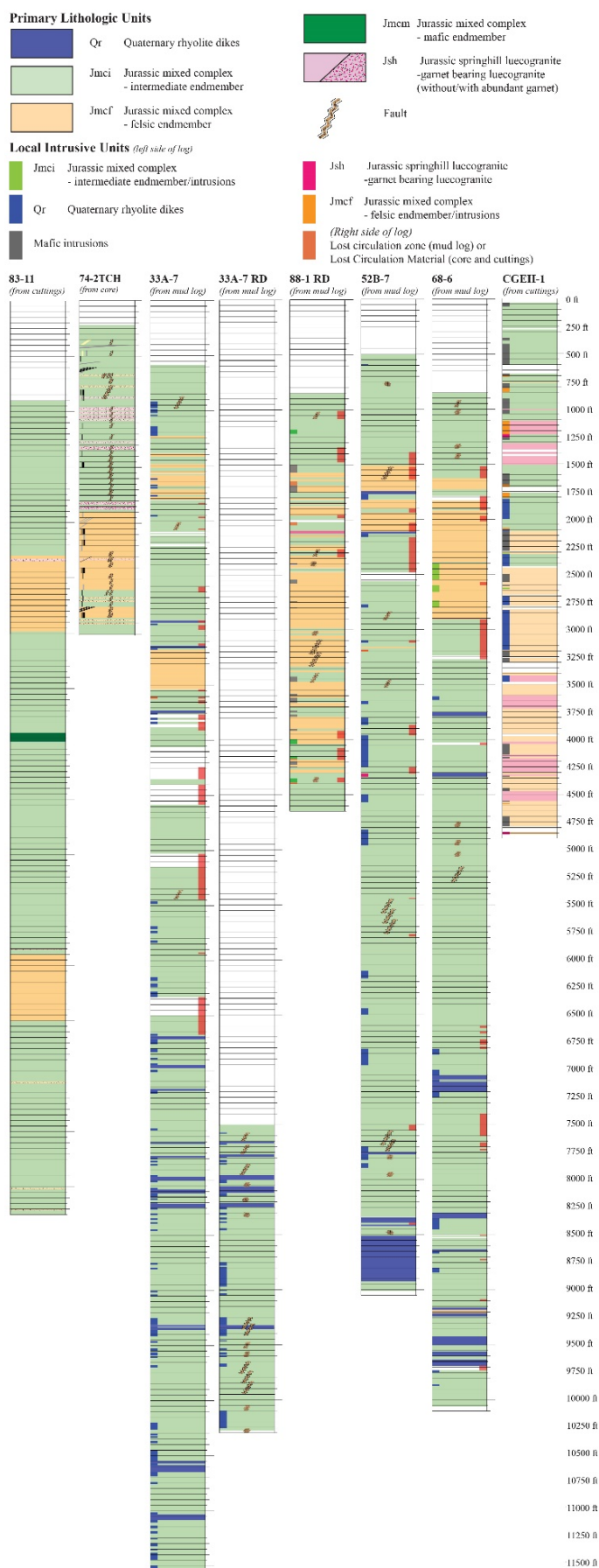
Figure 4. Lithologic logs of the eight wells used to characterize the subsurface lithology and structure at West Flank of Coso.
