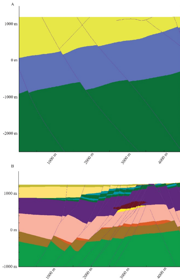
Figure 9. Cross-sections through 3D geologic models at (A) Fallon FORGE site, and (B) Brady's geothermal system (Siler et al., 2016). Both models were built with identical methods, similar data, and similar data density. The dense anastomosing fault system at Brady's hosts natural geothermal fluid flow at several intervals between elevations of ~1000 to -500 m. Faults at Fallon are widely spaced by comparison
