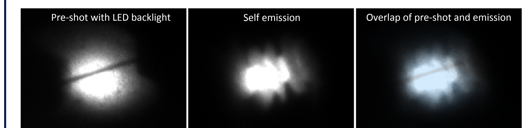
Relation of wire to emission for nickel wire at 380 ns machine time.
