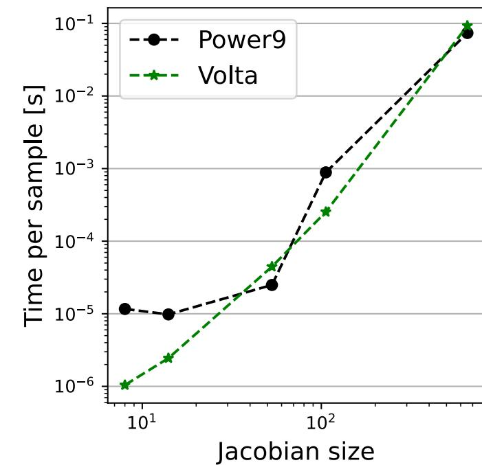
Due to limitations of GPU memory, the number of state vectors for large kinetic model cannot be increased.
