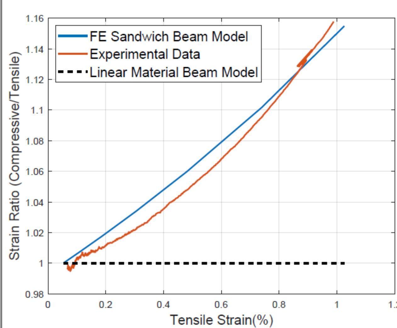
To validate the material model a model of the four-point bend test was developed and the strain ratio of the compressive and tensile faces while undergoing loading was compared to the experimental test. The virtual and experimental response showed good agreement. A linear material model is additionally shown for reference
