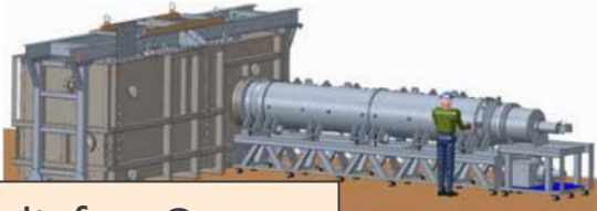
Fast Marx prototype and flashover test bed
