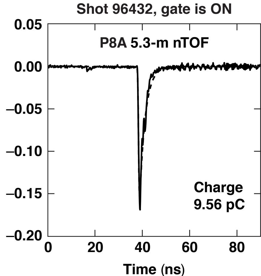
Only 7% (9.56/135.45) of hard x-ray signal is from direct interaction with the MCP inside the PMT.
