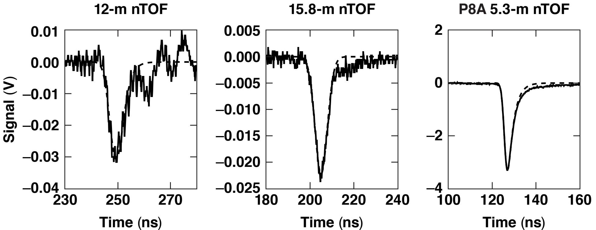
There are not enough nTOF detectors for low-yield DT in the range from  $1 \times 10^{11}$  to  $1 \times 10^{12}$  on OMEGA. The 12-m nTOF and 15.8-m nTOF have low neutron statistics and high electromagnetic pulse (EMP) noise below  $1 \times 10^{12}$ . The P8A 5.3-m nTOF detector will cover the DT yield range from  $5 \times 10^{10}$  to  $1 \times 10^{12}$ .
