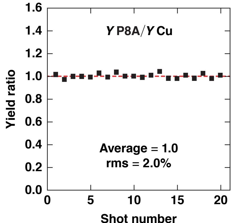
The P8A 5.3-m nTOF detector was calibrated in DT ion temperature against a 22-m nTOF Petal detector
