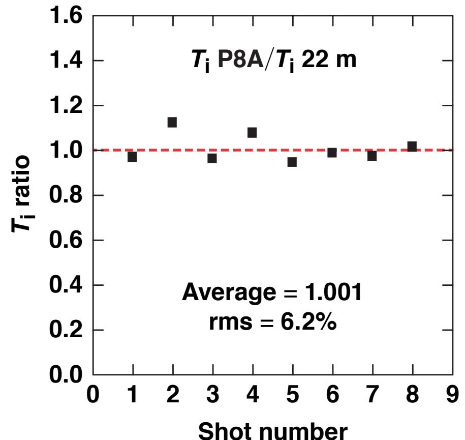
**A new nTOF detector designed for D<sub>2</sub> and low DT neutron measurements was installed and calibrated on OMEGA**
