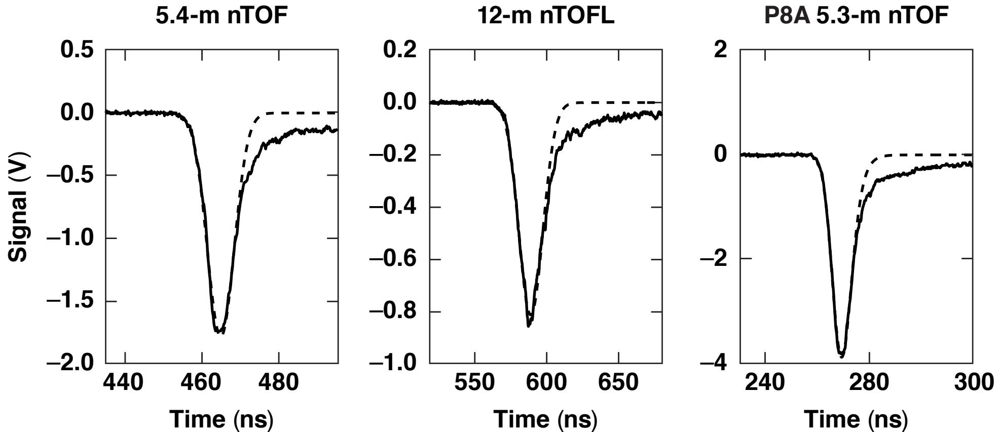
The P8A 5.3-m nTOF is more sensitive than the 5.4-m nTOF and 12-m nTOFL detectors.
