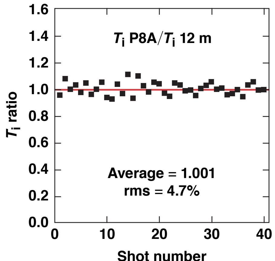
The P8A 5.3-m nTOF detector was calibrated
