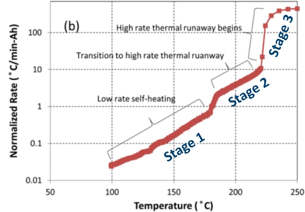
Initial low-rate self-heating as electrolyte breakdown, SEI dissolution begin
