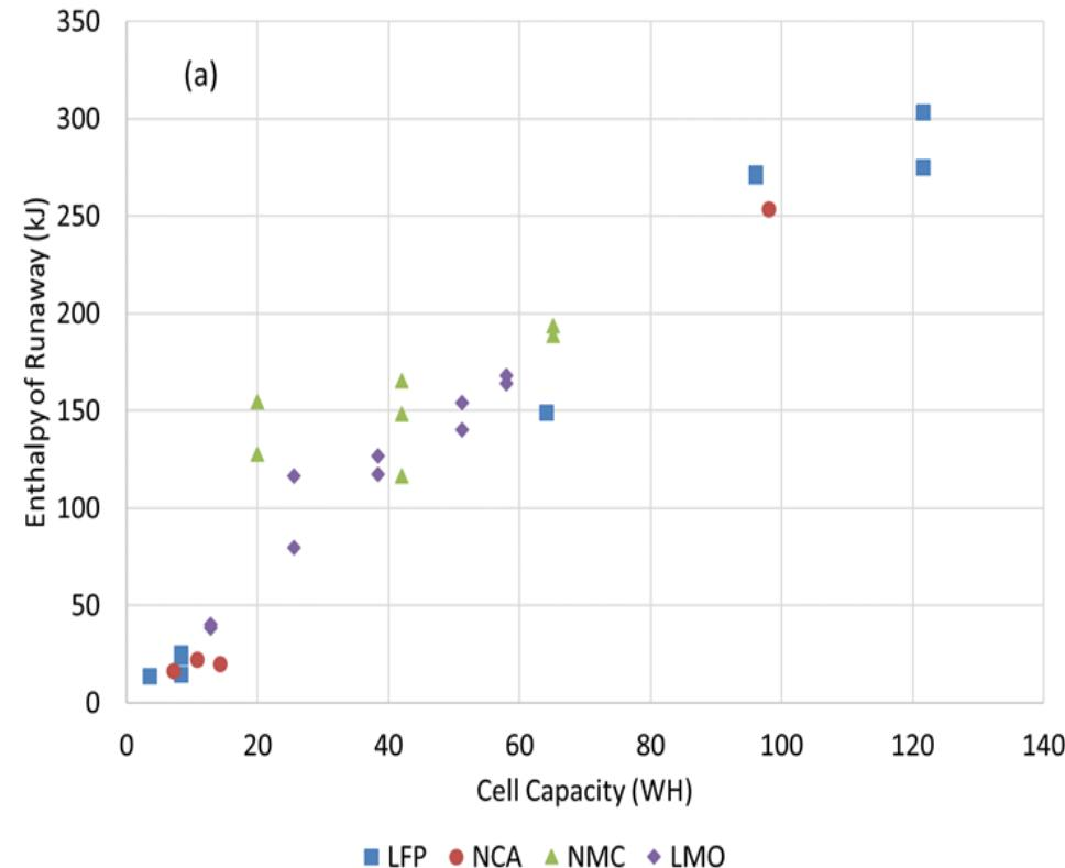
Total energy of runaway maintains a linear relationship to cell capacity
