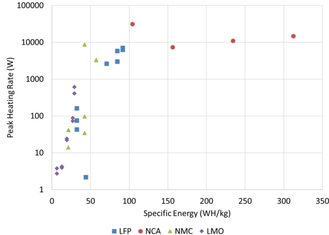
Logarithmic behavior up to very high specific energies - Ability of equipment to evaluate very high peak heating rates is limited- the flat line behavior at this point may be because of this
