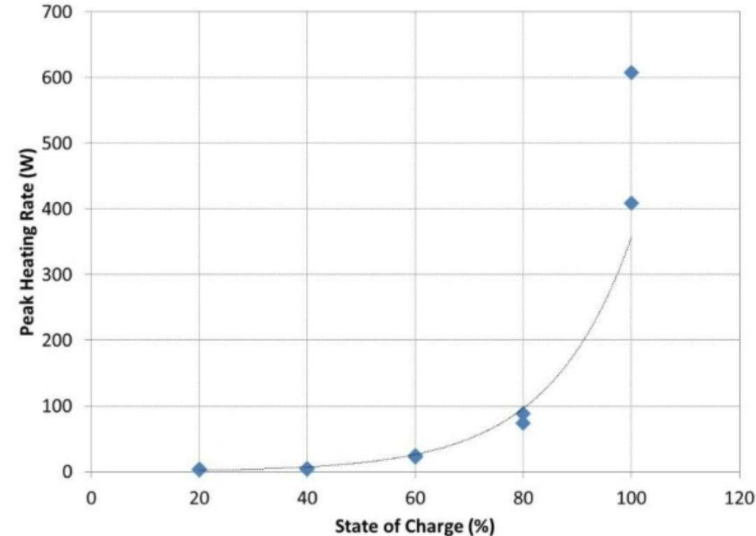
Heat release rates (e.g. runaway reaction kinetics) follow an almost exponential relationship with cell SOC
