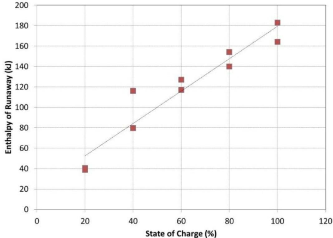
Nearly linear relationship between total heat release (kJ) and cell SOC – failure enthalpy is based largely on the stored energy available
