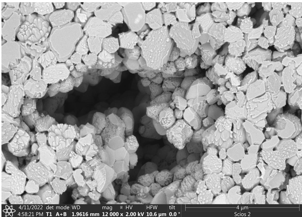
Backscattered electron image of cavity in alumina after etching to reveal grain facets. Image collected on a Scios 2 DualBeam focused ion beam scanning electron microscope (FIB-SEM).
