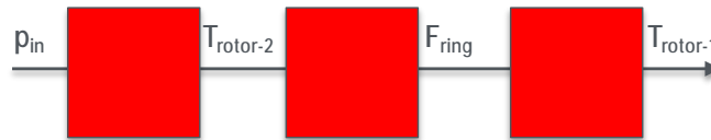
Figure 17. Block diagram for conversion of pressure differential to rotor torque.
