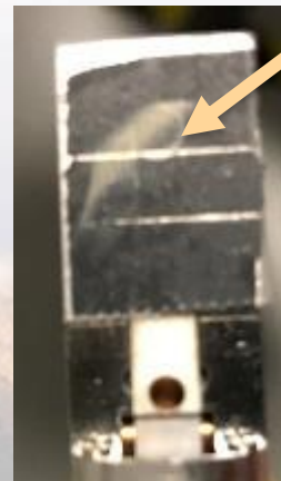
He beam is only partially covering 3mm circle—may have been lower current at imaging location than measured in FC
