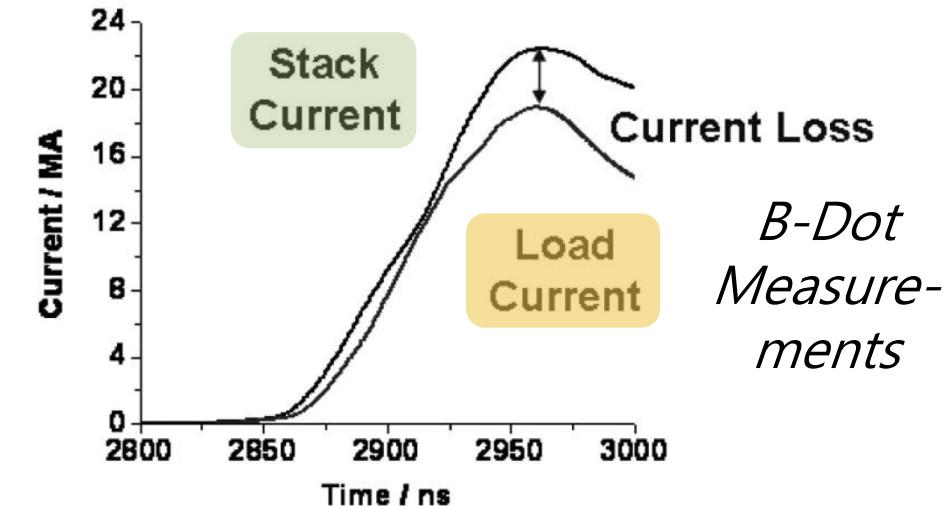
Previous work focused on current loss due to plasma formation in the convolute.
