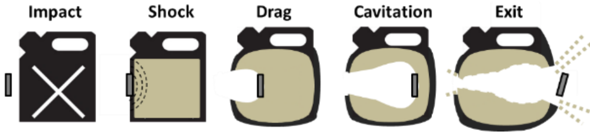
Figure 1 Hydrodynamic ram on a fuel tank illustration.
