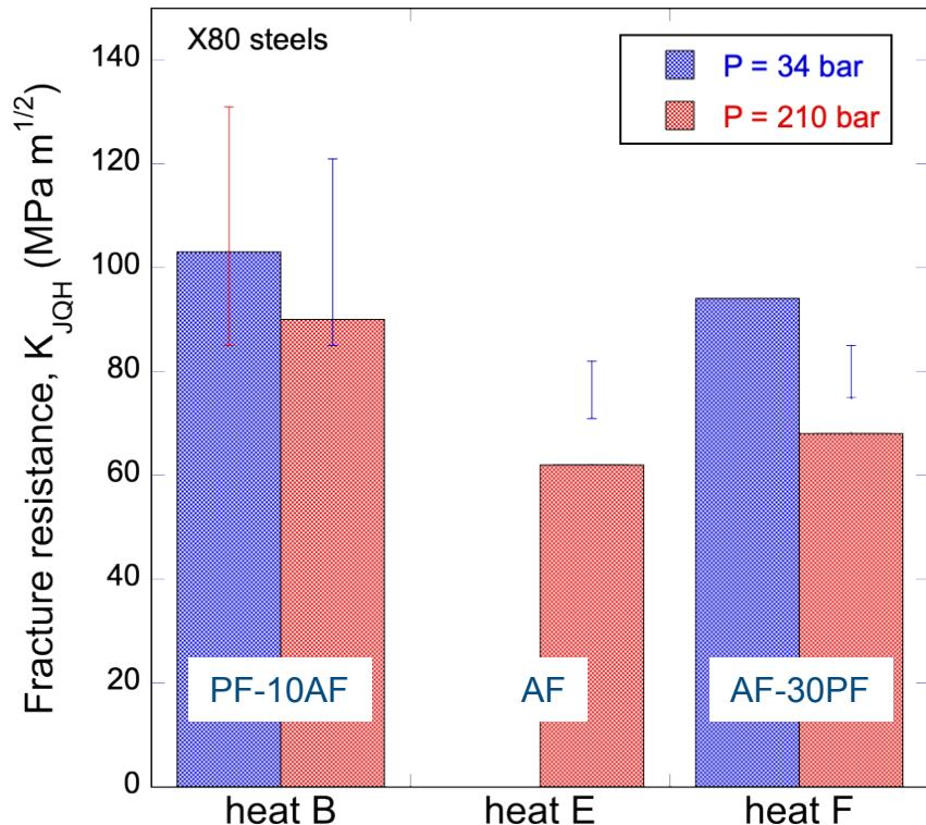
ASTM E1820 elastic-plastic fracture measurements at the conclusion of fatigue testing
