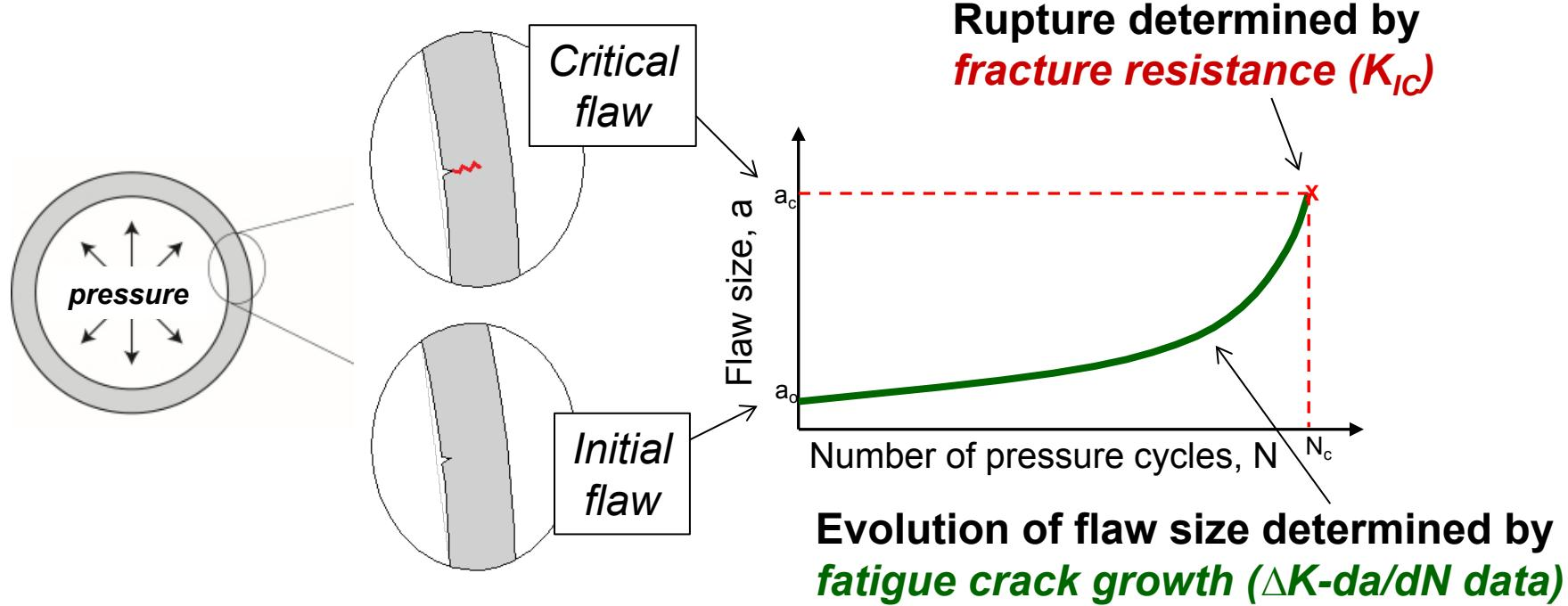
ASME B31.12 describes rules for hydrogen pipelines with reference to ASME BPVC Section VIII, Division 3, Article KD-10
