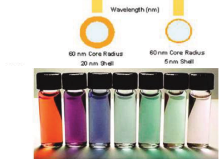
SiO 2 coated gold with varying shell widths producing different optical resonances 1 .
