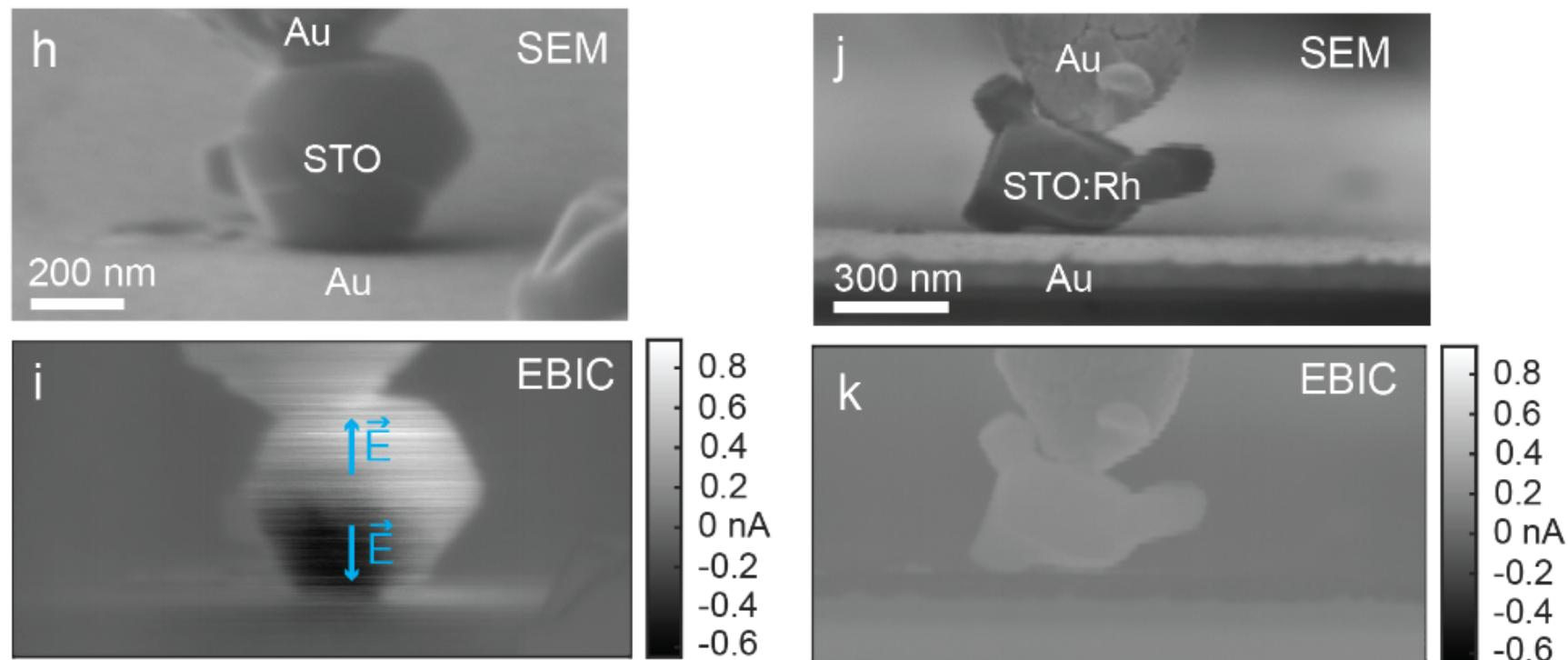
No significant built-in E field, no free carriers to screen changes in work function
