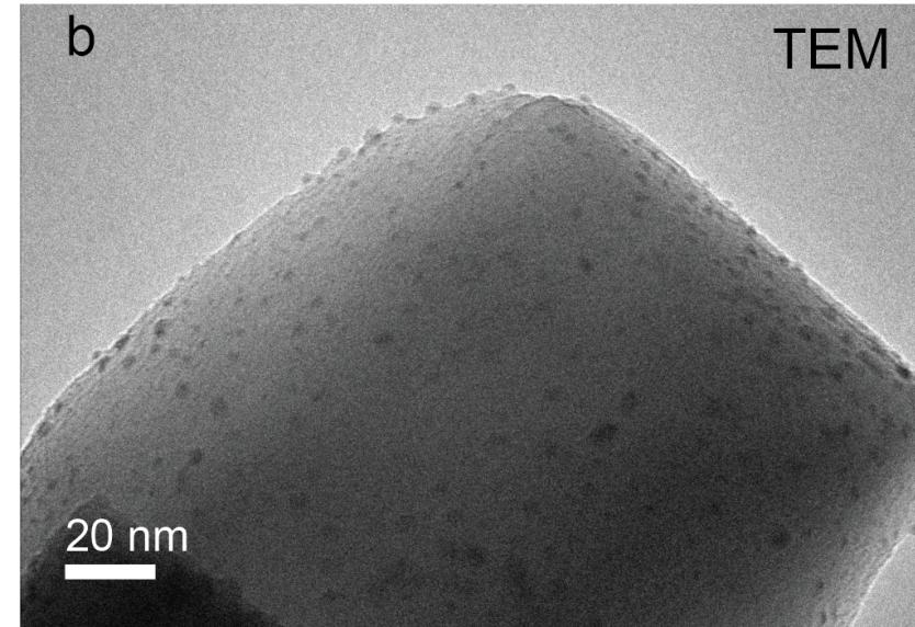
Electrostatically, a Pt co-catalyst of 5 nm diameter can have a depletion region of, at most, 10-15 nm
