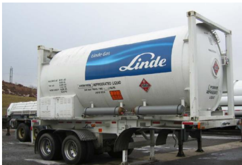
LH 2 Storage Tank on Trailer
