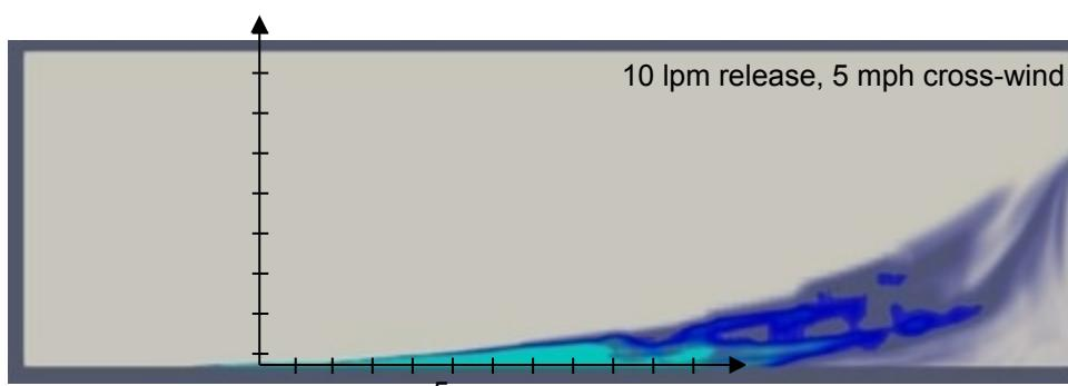
Simulated concentration of hydrogen downwind of the release for different experimental conditions
