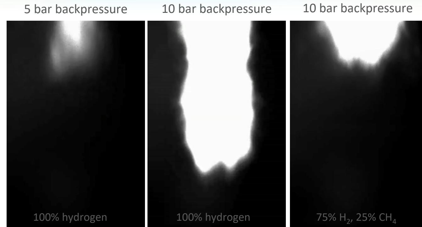
Chemiluminescence of laser spark ignition of gases through a 1mm diameter nozzle (15/1000 speed). Pure hydrogen at moderate pressure (left) and 25% CH<sub>4</sub> (right) show flame blow-off while pure hydrogen at a higher pressure (center) ignites into a jet flame.
