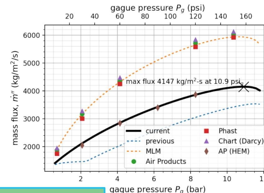
Calculations are repeatable in several implementations. Current calculation (black line) has increased flux over previous (blue dashed) but is less conservative than metastable liquid model (MLM).
