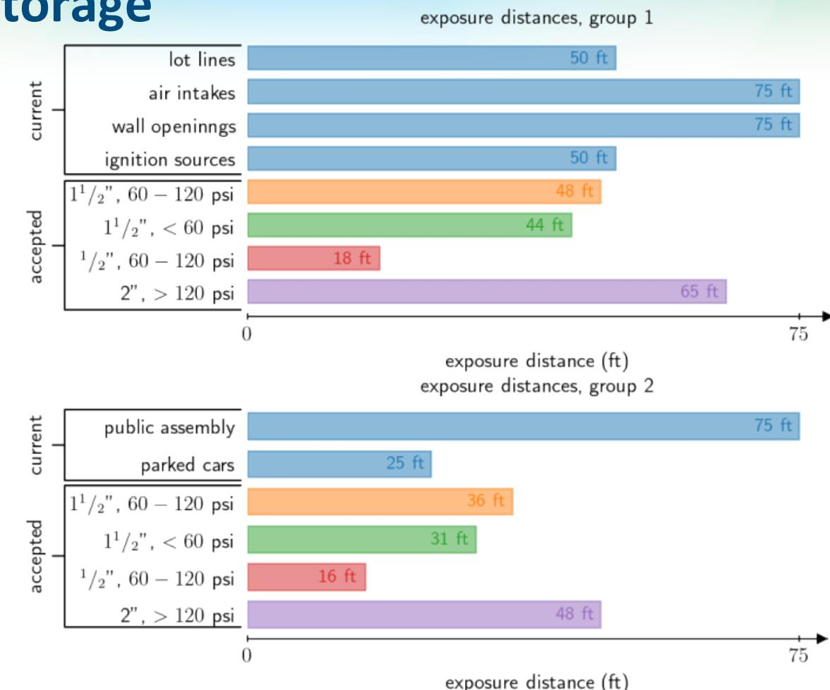
➤ Most distances reduced for typical pipe size (1.5") and operating pressure (vs typical tank volume); some increase (but mitigations, i.e. walls can be used)
