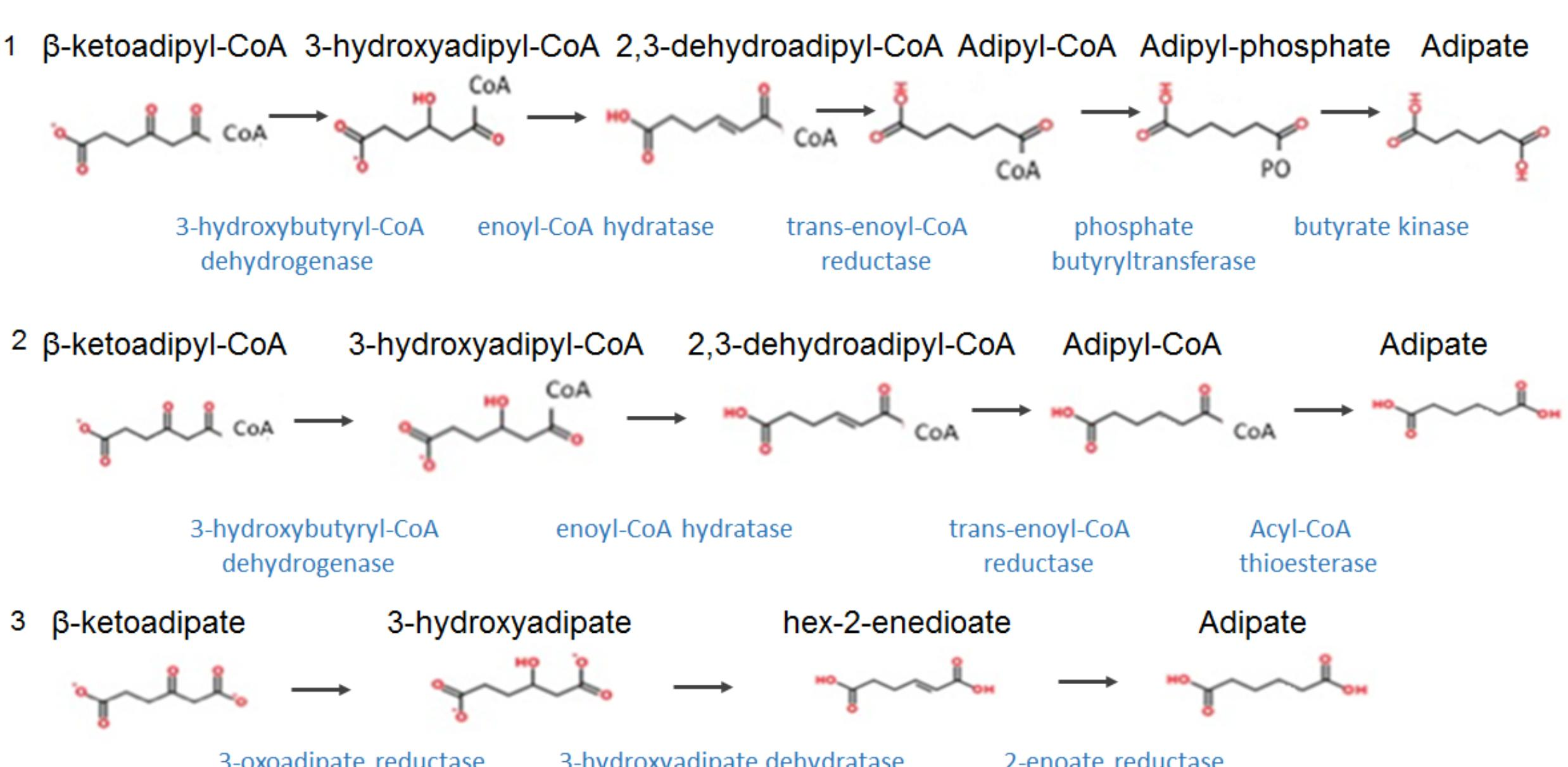
Three adipic acid pathways were designed to utilize intermediates from the native  $\beta$ -ketoadipate pathway. Strains were developed that can generate these intermediates from either aromatics or sugars derived from lignocellulose.
