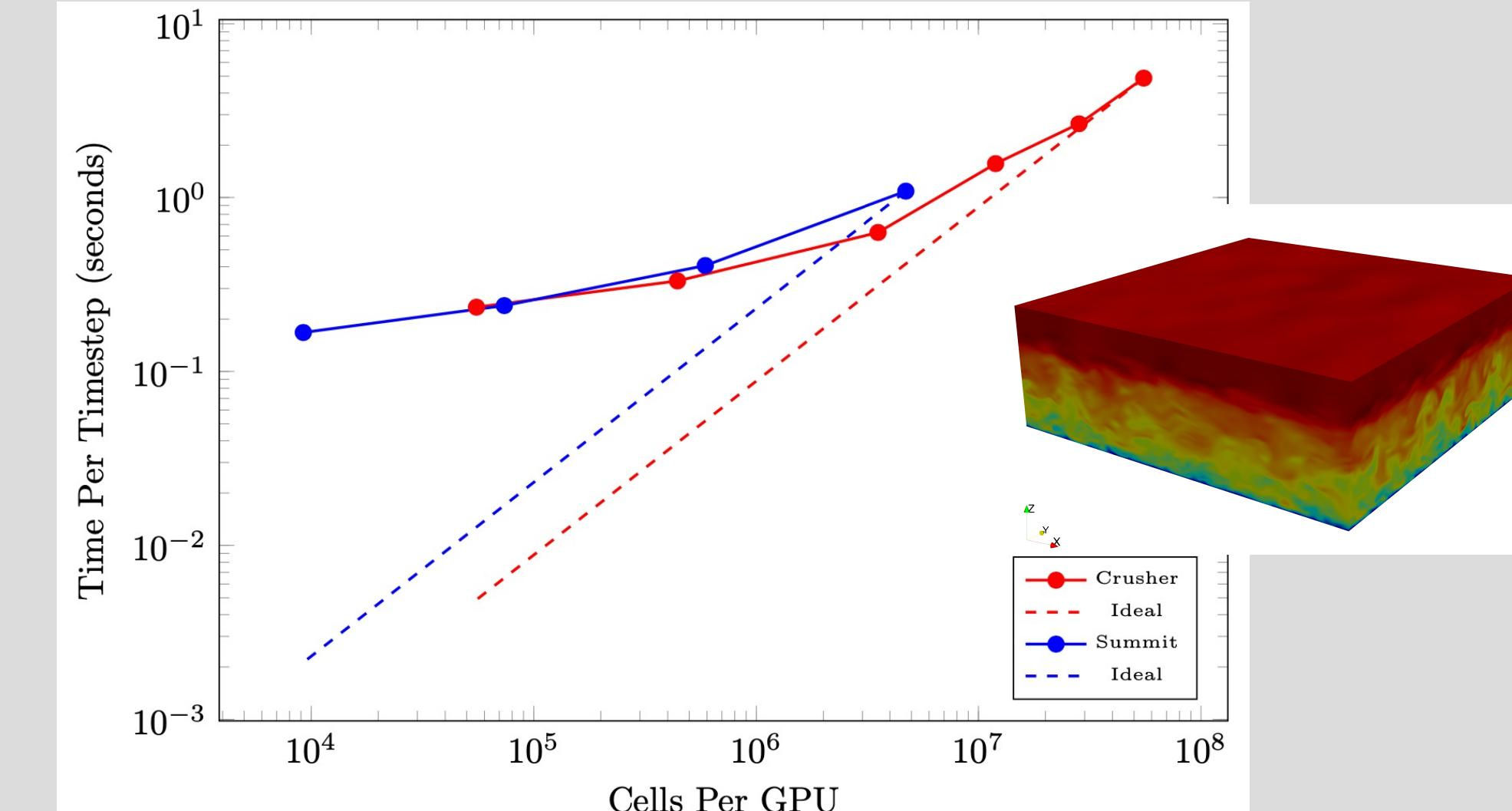
Scaling plot comparing AMR-Wind performance for atmospheric boundary layer simulations on Summit and Crusher GPUs. Simulations of different model sizes were run on a fixed resource of 16 Crusher nodes (128 GCDs) or 16 Summit Nodes (96 GPUs). The largest models were  $1920^3$  and  $768^3$  on Crusher and Summit, respectively.
