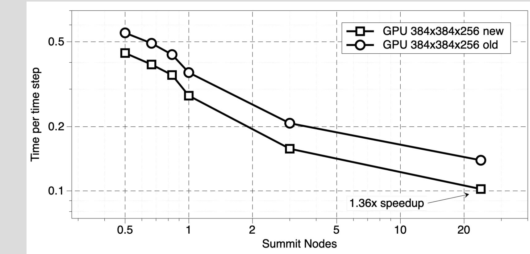
Strong scaling results on Summit GPUs for an atmospheric boundary layer simulation; "old" is from AMR-Wind in April 2021, whereas "new" is AMR-Wind in April 2022.
