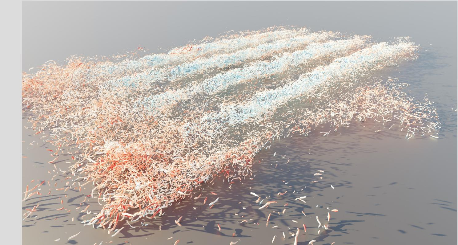
AMR-Wind Summit simulation results for a 20-turbine wind farm off the coast of NY, where wind turbines were represented as "actuator lines". Shown are iso-surfaces of  $q$ -criterion colored by velocity magnitude. (Figure: S. Yellapantula)
