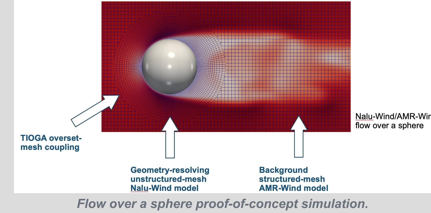
Flow over a sphere proof-of-concept simulation.
