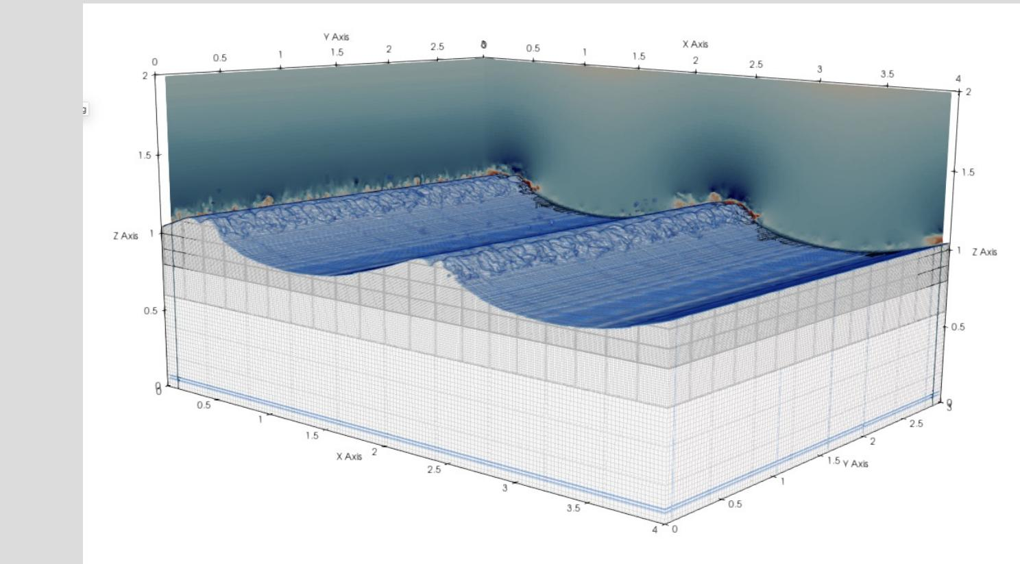
Multi-phase flow simulation of waves in AMR-Wind (Figure: Georgios Deskos)
