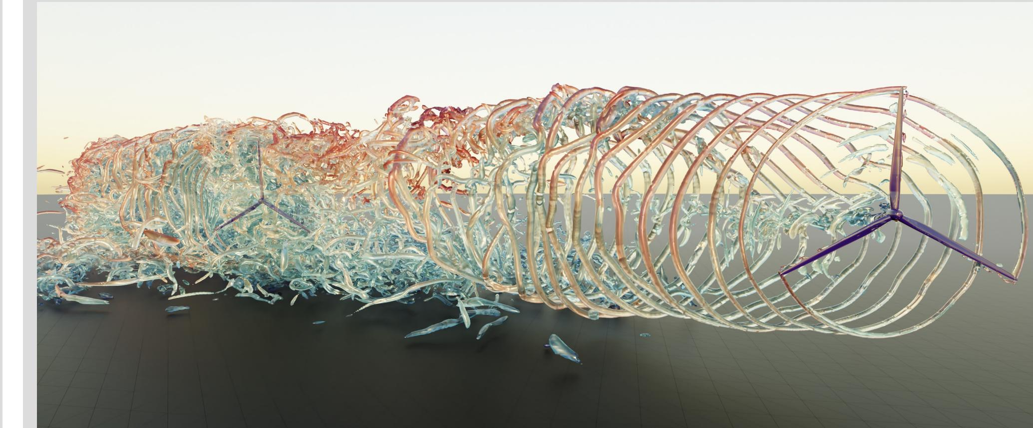
Representative two-turbine blade-resolved simulation with the ExaWind hybrid solver on NREL's Eagle computer. The near-body flow is resolved with an unstructured-grid Nalu-Wind model and the background flow is resolved with a structured-grid AMR-Wind model. The models are coupled through overset meshes handled by the Topology Independent Overset Grid Assembler (TIOGA).
