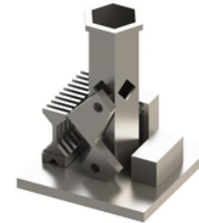
Figure 7. An example witness artifact that enables rapid measurement of 11 material properties in a compact footprint.
