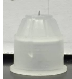
Assembled device with capillary for fluid storage
