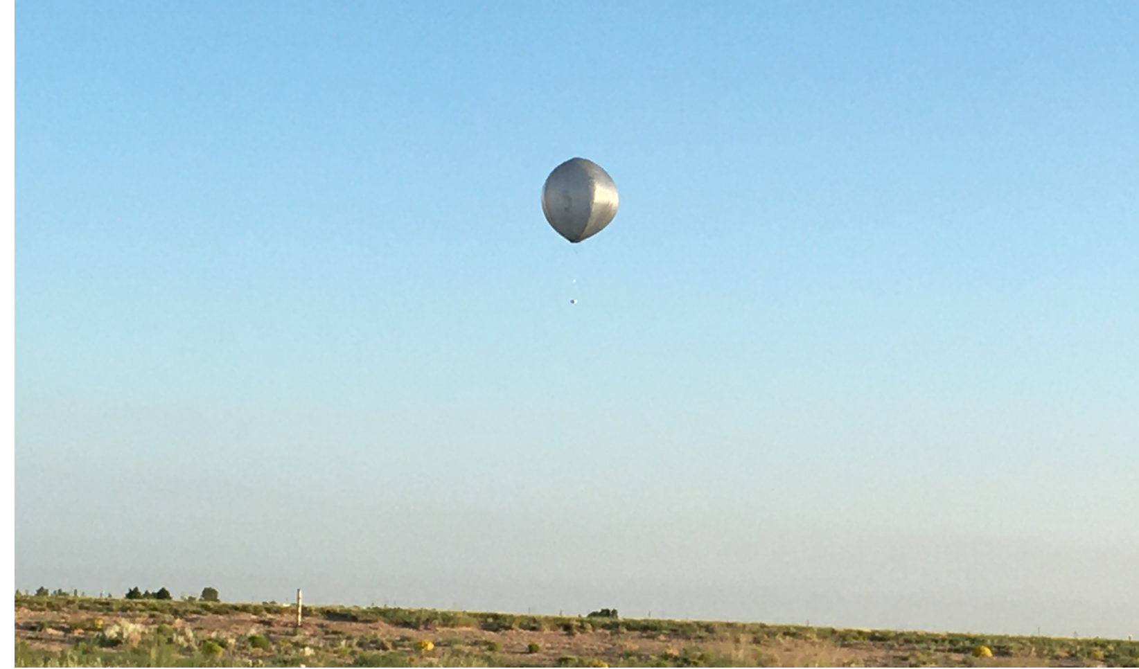
Figure 1: A solar hot air balloon with an infrasound payload moments after launch.
