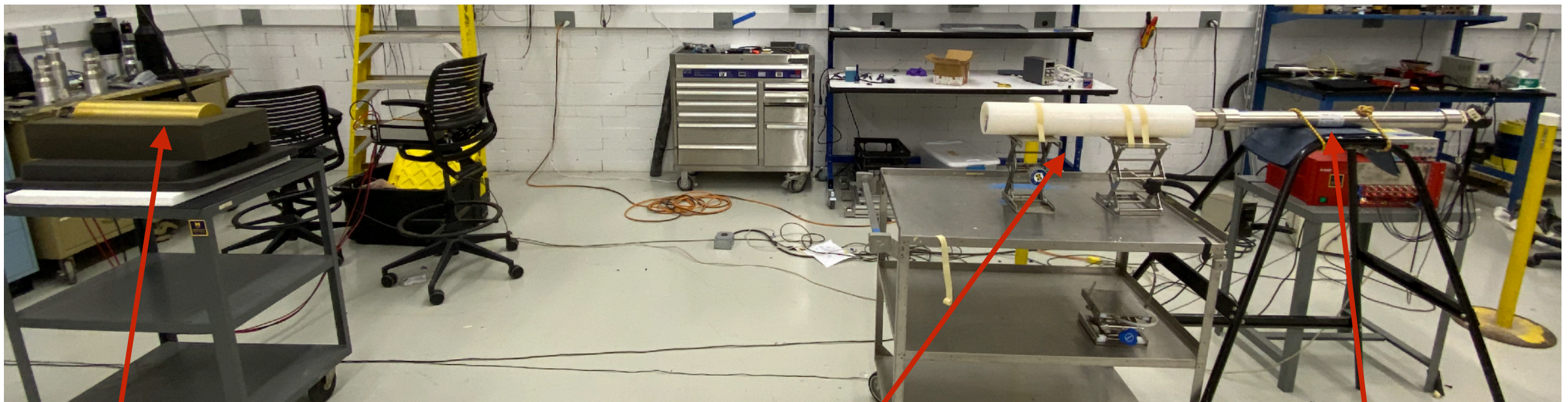
^4\text{He} scintillation detector
