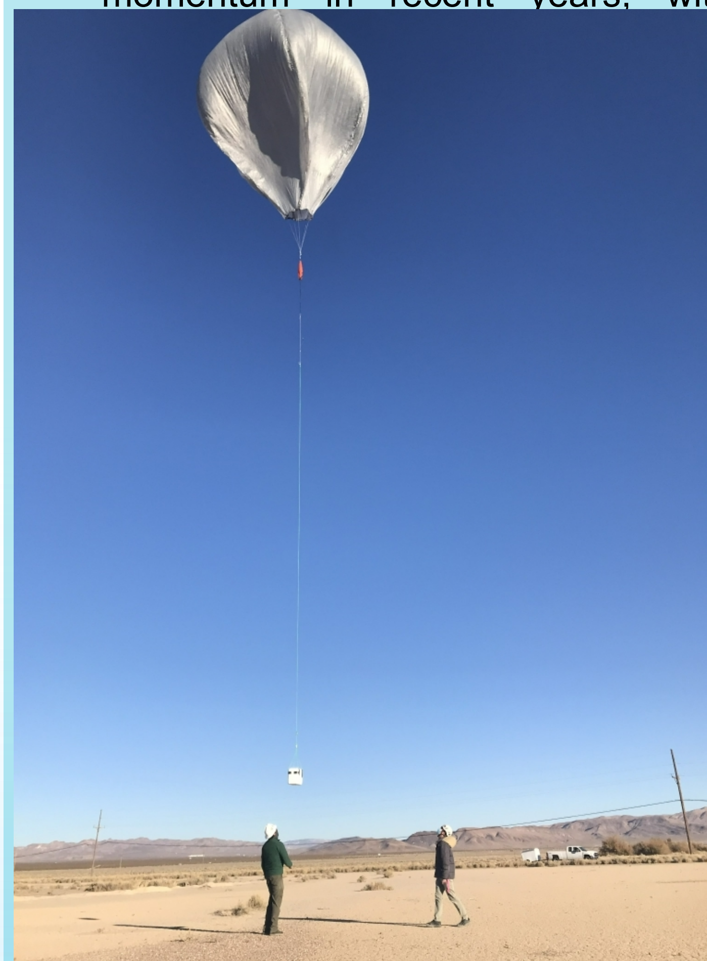
Figure 1: High altitude balloon launch. The balloon is shown as it is starting to ascend. Payload is attached via paracord.
