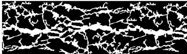
Reconstructed multi-scale porous material
