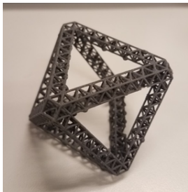
Figure 58: Hierarchical multiscale structure of octahedral (second-order). Printed in Georgia Tech Invention Studio.
