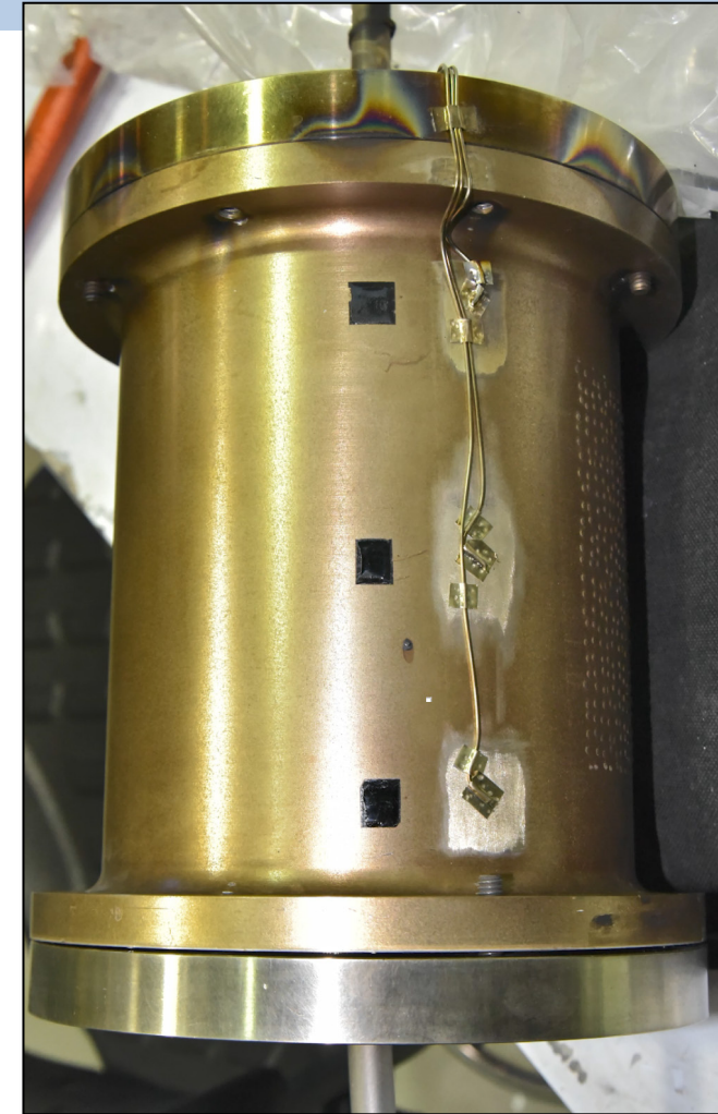
post-test scan showing leak pattern at top endcap, and survival of welded external TCs and Ta pattern
