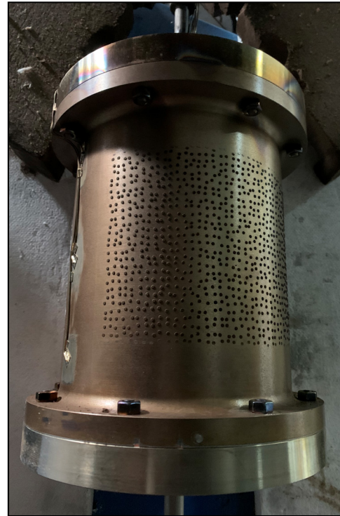
post-test with x-ray DIC
