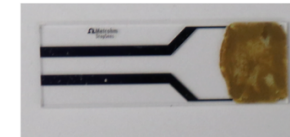
IDE + Ni-MOF-74 Exposed to 5ppm NO 2 8 h 50 °C
