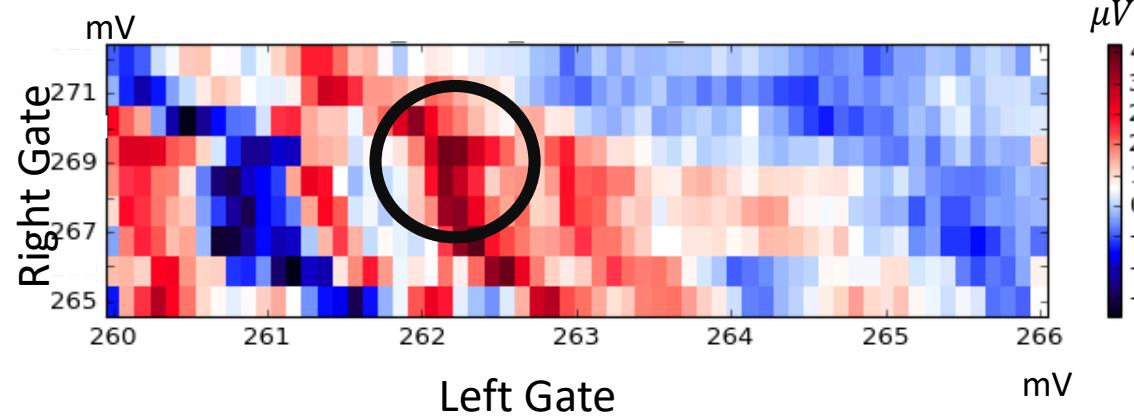
Coulomb drag scan, voltage in drag wire is measured as wires are varied. Circle indicates peak tracked for T dependance
