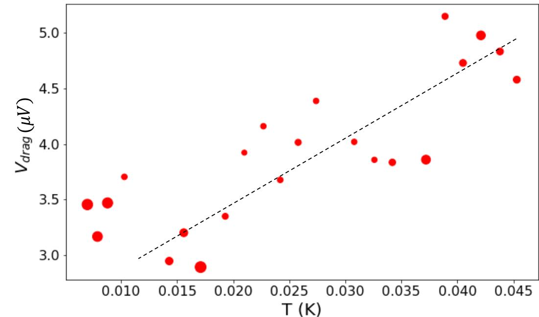
Tracking the strongest peak as a function of temperature. Thermal trend seems to confirm that we have achieved cooling down to at least 15 mK
