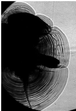
Fig. 5. Monoblock unstressed shadowgraph at 600 \mu s
