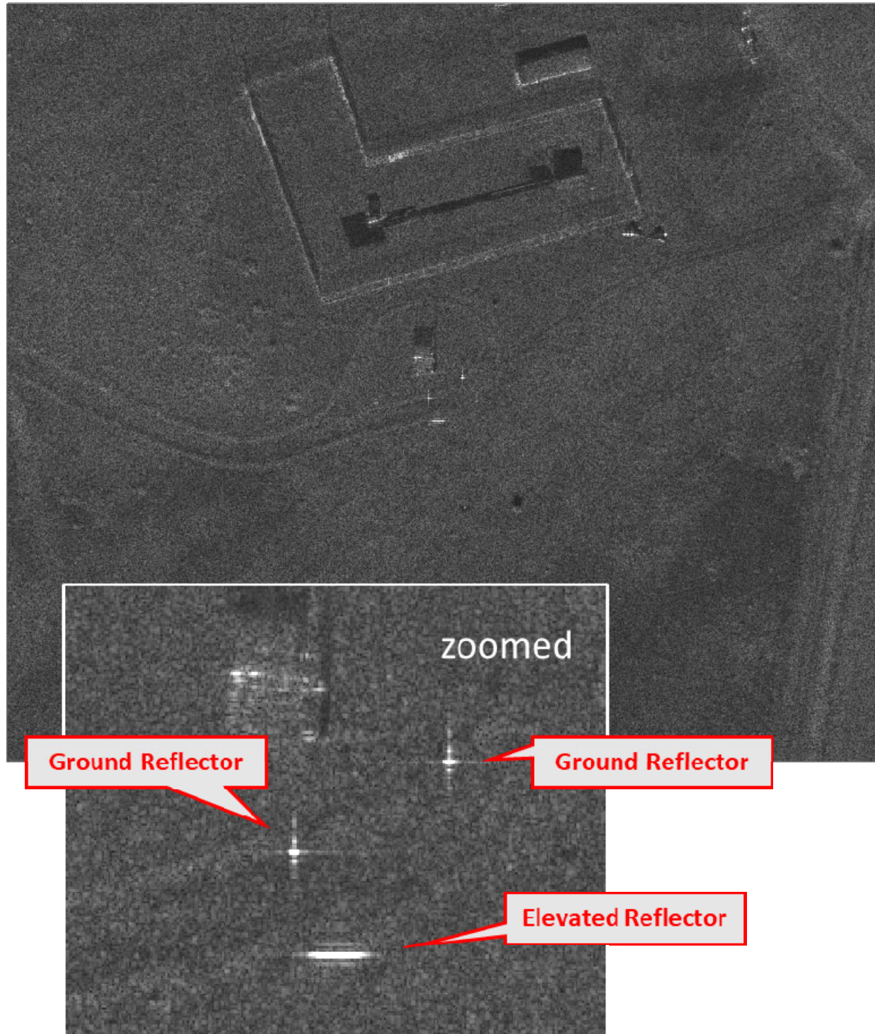
Figure 5. Example of defocusing due to elevated target reflector. Elevated reflector is on a pole about 16 m above the ground. Image was collected with a Sandia Ku-band testbed radar, flying an approximately circular orbit flightpath, operating at 4 km range, 29.8 degree grazing angle, 0.1 m resolution. Scene is of a facility on Kirtland AFB, Albuquerque, New Mexico, USA. HOF is calculated to be about 3.33 m.
