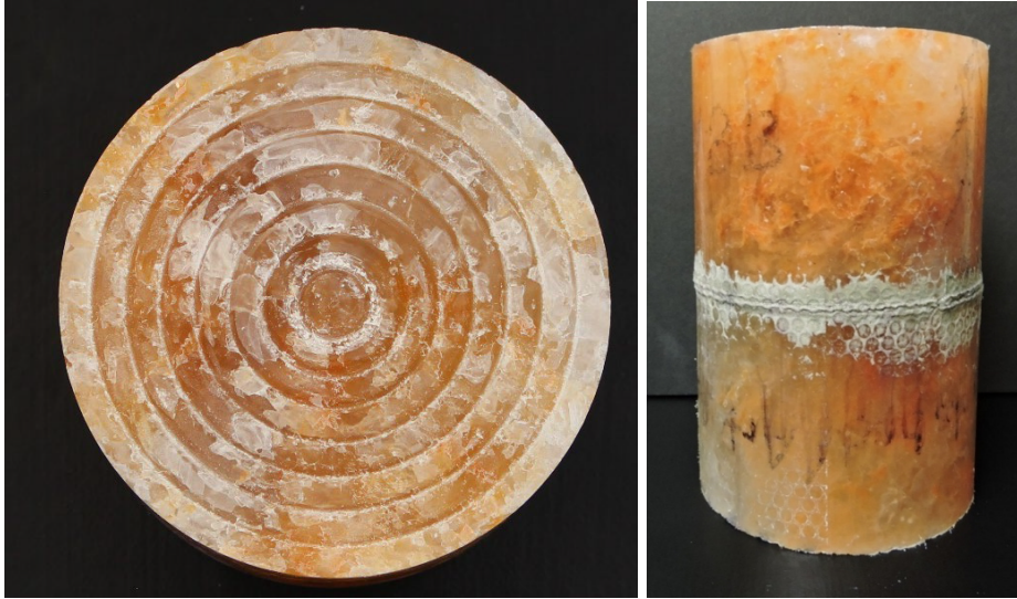
Figure 3. Photographs of grooves machines into salt sample, and consolidated test specimen.
