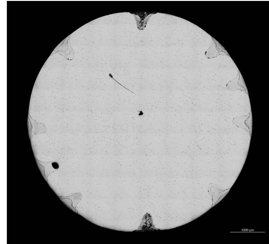
Step 3: Section welds in transverse, scan HAZ for cracks
