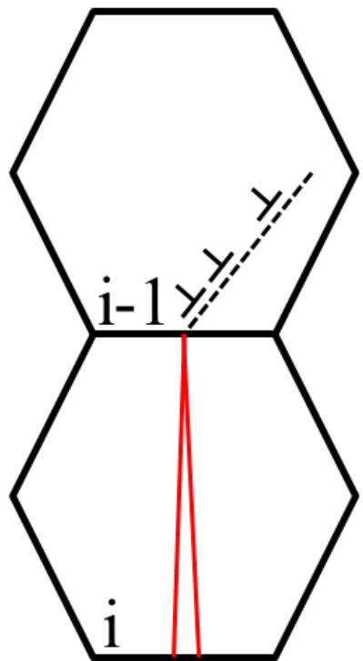
Crack Termination: Hard Grain
