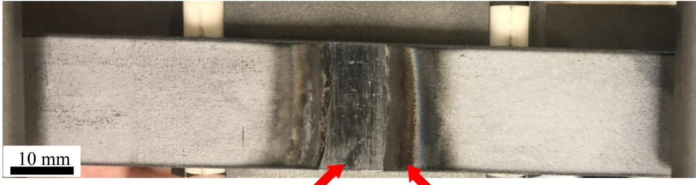
Result after 17 hours of corrosion
