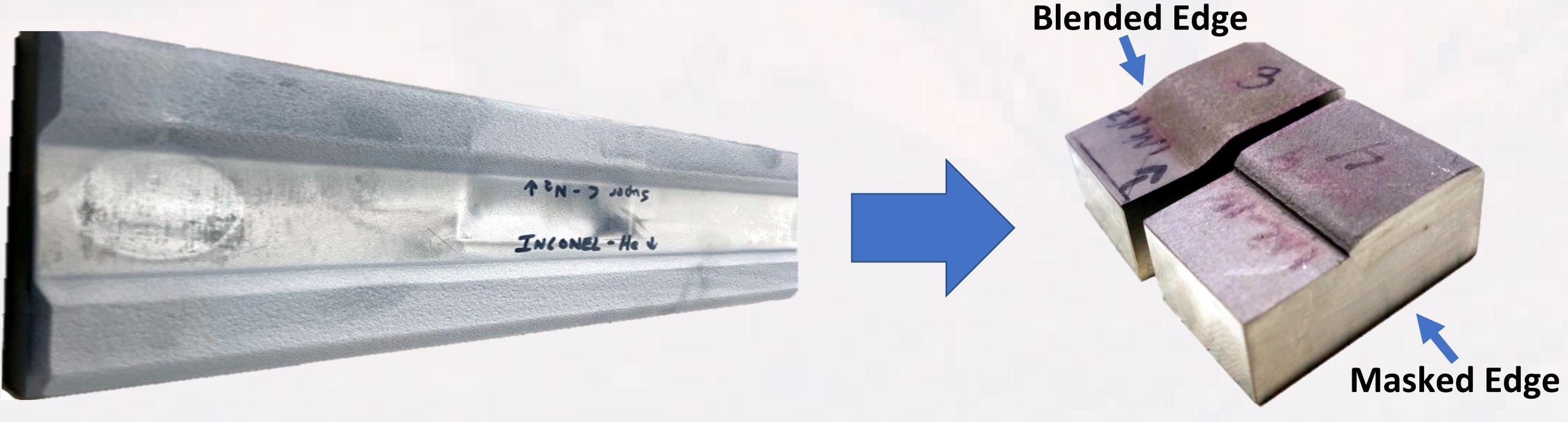
Single alloy cold sprayed plates and samples.<sup>1</sup>
