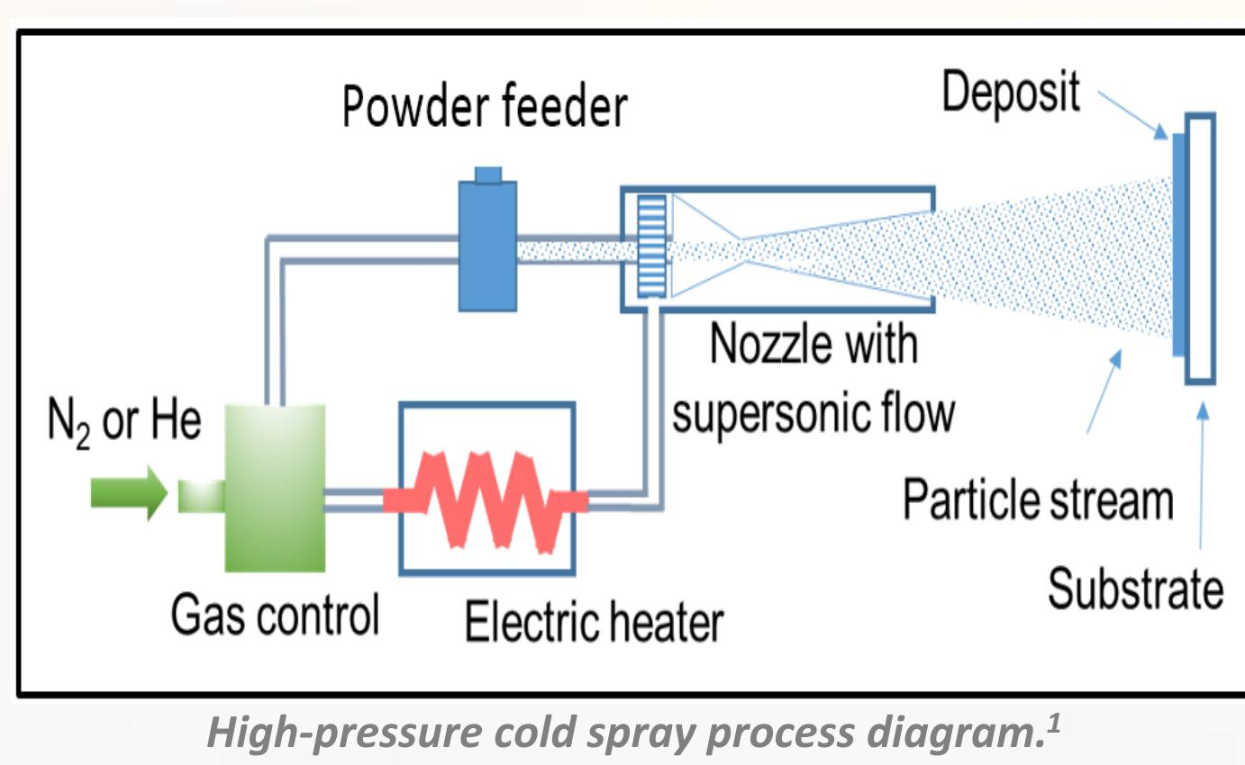
High-pressure cold spray process diagram.<sup>1</sup>
