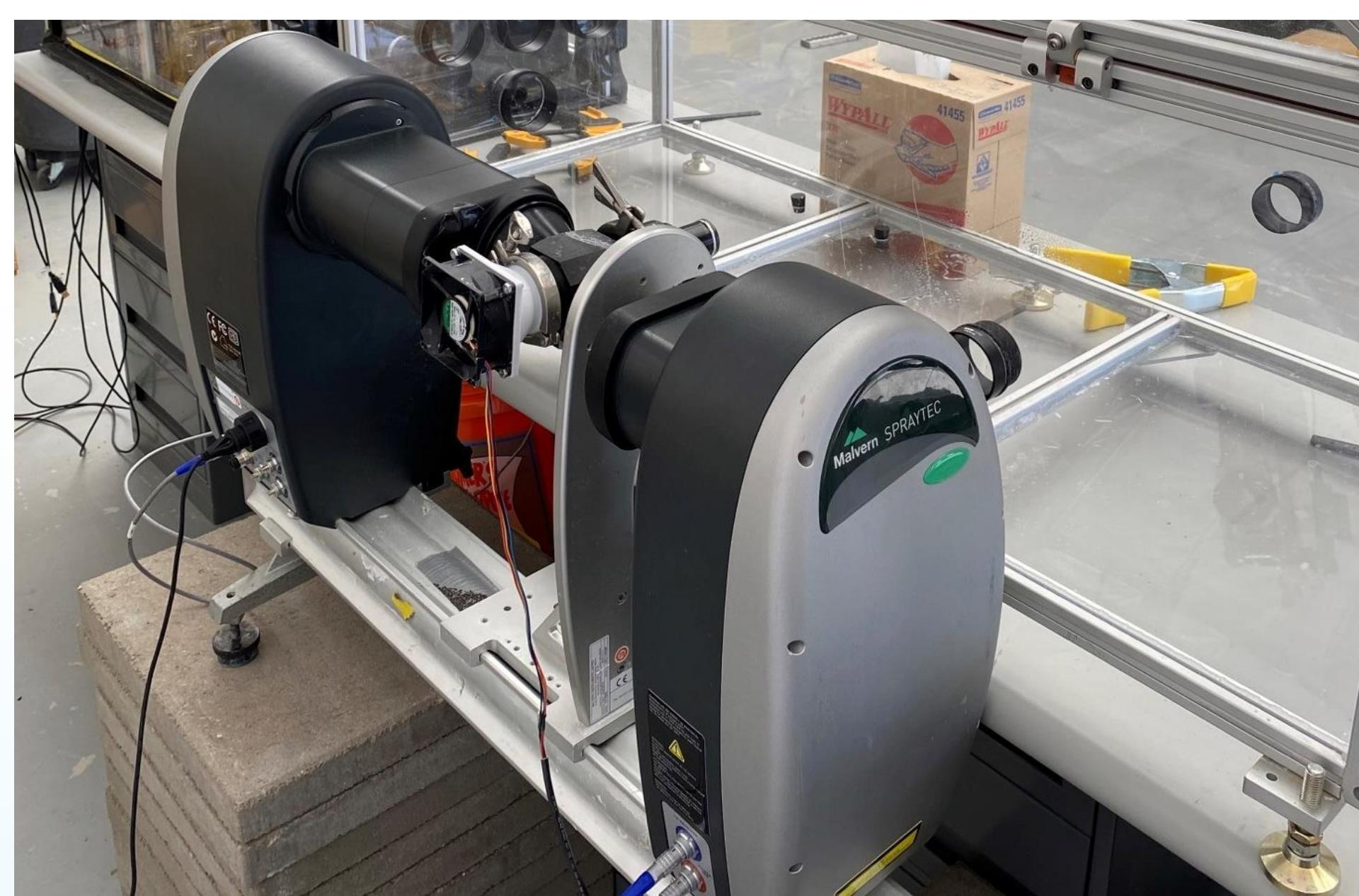
**From top to bottom:** super-resolution imaging test, transmissometer visible (green) and experimental (red) beams can be seen scattering; side-by-side images of different fogs generated by the chamber; Malvern Spraytec attached to the chamber
