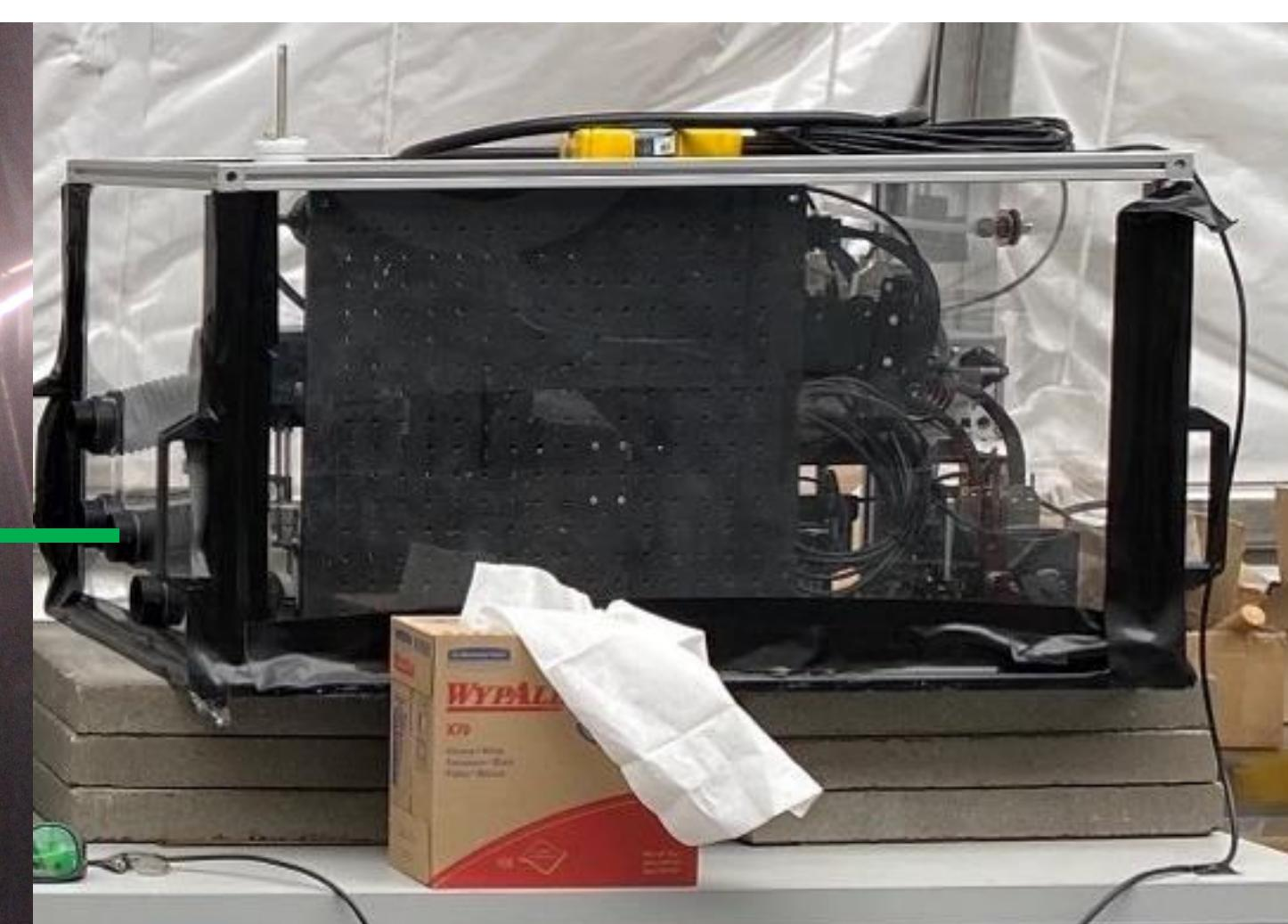
Malvern Spraytec, used to size fog particles.
