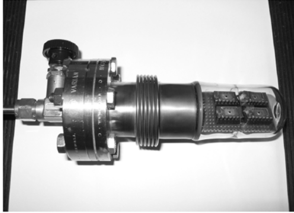
Fig. 2. Glass chamber flange used for soaking and radiation testing of samples under hydrogen environment [16].
